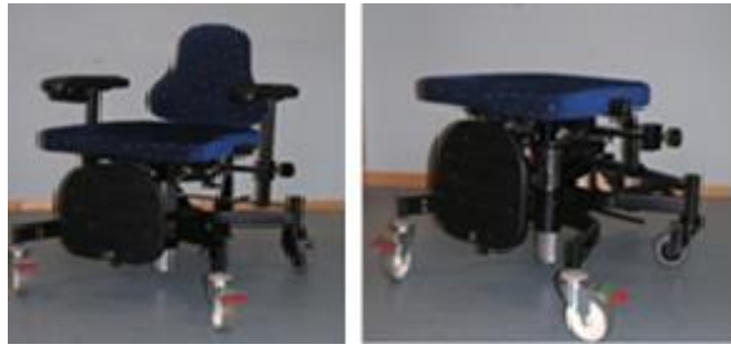
Figure 6 a) A chair with armrests and backrest, and b) a stool after removing armrests and backrest used during muscle strength measurements.
