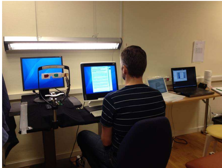
Figure 14. Illustration of the setup using a luminaire in front to induce direct glare when performing reading task in study IV.
