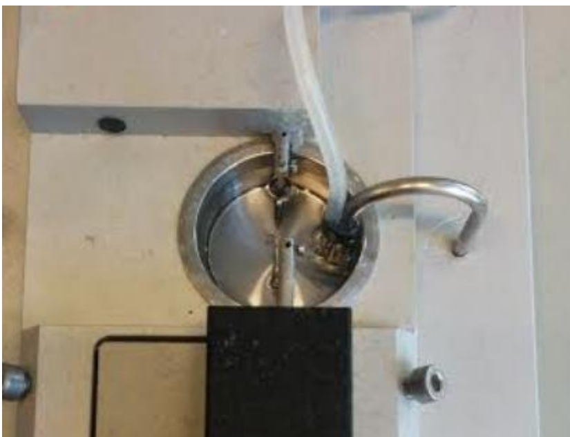
Figure 13 An organ bath with a bronchial segment mounted between the metal prongs in the centre.
