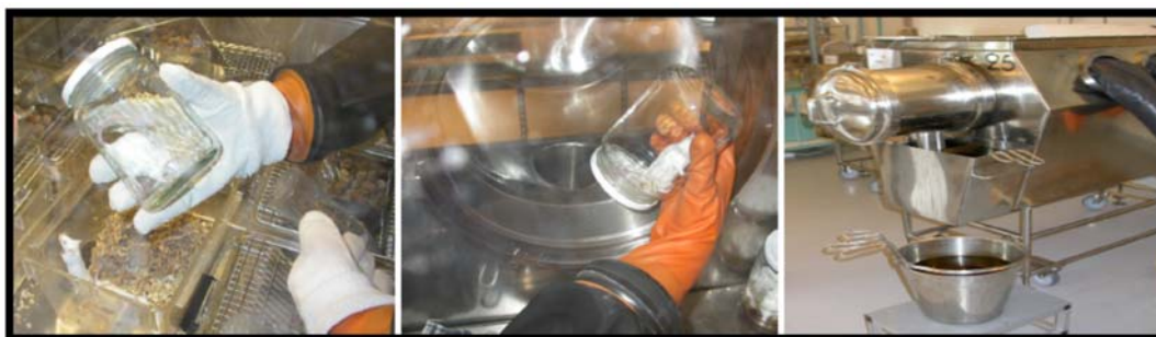
Figure 3.3 Transfer of mice from inside the isolator. The mouse is placed in an autoclaved glass jar and transferred through a sterilized lock into the tank filled with disinfectant.
