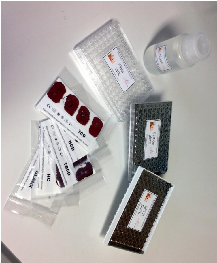
Figure 2. SCREEN-ID kit-like assay version for quantitative analysis of (i) TREC-KREC-ACTB or (ii) TREC-KREC-UNC13Dwt copies in neonatal DBS. The kit consists of pre-arranged 96-well plates containing a DNA-elution solution in the ‘Elution plate’, and qPCR reagents and plasmid standards for real-time qPCR in the ‘qPCR plate’; both plates can be stored frozen at -25^{\circ}\text{C} for up to 6 months. Only a single pipetting step is required to wet DBS with a rinse solution in the ‘Filter unit’. All further assay steps rely on centrifugation of the plates containing DBS and assay reagents. Control card specimen are allocated to mimic T-cell deficient (TCD), B-cell deficient (BCD) or T- and B-cell deficient (TBCD) patient samples.
