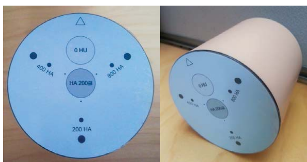
Figure 8. Cardiac CT Calibration Insert Phantom for the Quantification of Coronary Calcium (QRM, Möhrendorf, Germany).
