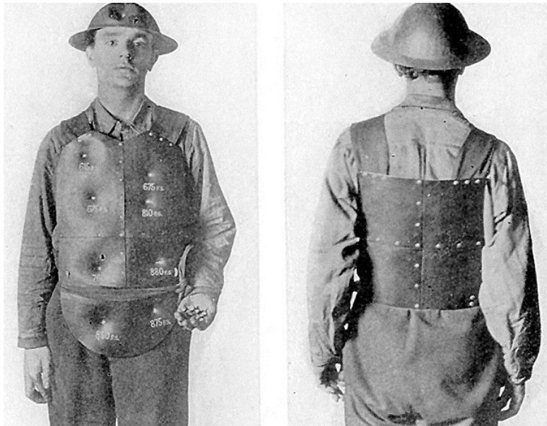
Figure 1. British Dayfield body shield (front and rear view) (reproduced from “Modern body armour and helmets: An introduction”, with permission from Michael Iremonger).
