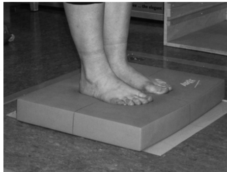
Figure 5. The foam surface provided by an Airex® Balance-pad placed in the center of the force platform.
