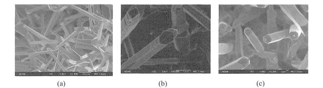
FE-SEM images (a), (b), and (c) are for  $In_2O_3$  nanostructures deposited on a substrate placed at the center of the heating furnace at temperatures of 700, 800, and 900 °C, respectively.
