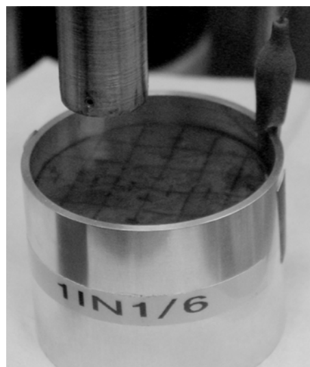
Fig.3 Photograph of PIN-diode and coring specimen
