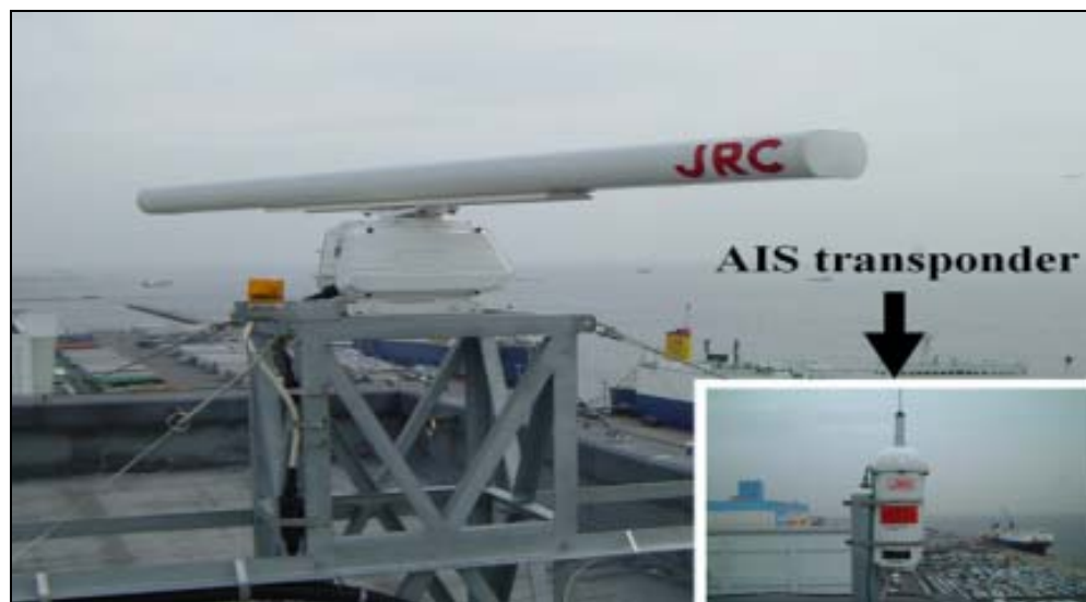
Fig 2 10 AIS transponder and radar antenna of Kawasaki station
