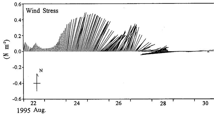
Fig. 7. Time series of 25-hours running averaged wind stress (Newton/m<sup>2</sup>) at Tateyama. Each wind stress vector indicates the direction toward the wind blowing.
