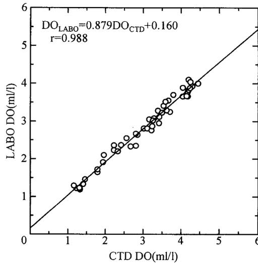
Fig. 2. Comparison of the dissolved oxygen obtained by CTD (CTD DO) and that measured by Winkler's method (LABO DO). Solid line is a regression line.
