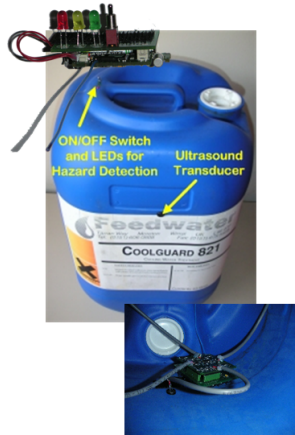
Fig. 2. Chemical container instrumented with Particle Smart-its.
