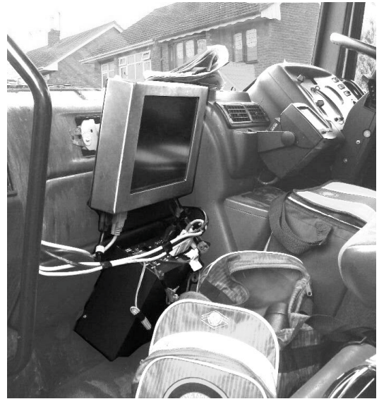
Figure 6: The In-Vehicle computer
