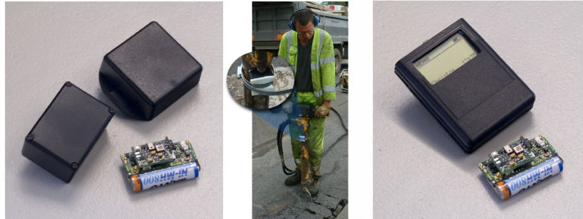
Fig. 3. Sensor-based vibration monitor system with wireless drill & dosimeter (reproduced from [7]).
