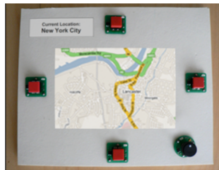
Figure 1. VoodooFlash provides a physical stage for interface prototyping(right) alongside the Adobe Flash’s virtual stage (left).
