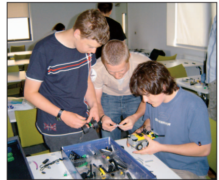
Figure 2. Team members collaborate on an iteration of their design. They're aiming to engineer a stable, speedy robot using a low center of mass and a relatively low gearing ratio.
