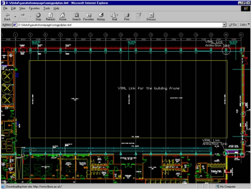
FIG. 8: 2D plan for the swimming pool with hyperlinks to VRML models and 3D animations
