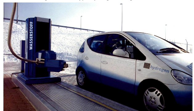
Fig 14: Prototype hydrogen filling station
