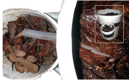
FIGURE 2: Plan view of a tunnel trap showing a mature L. terrestris exiting a 20-litre mesocosm into the attached 1-litre capture pot (lids removed). Insert shows a lateral view of the whole setup.
