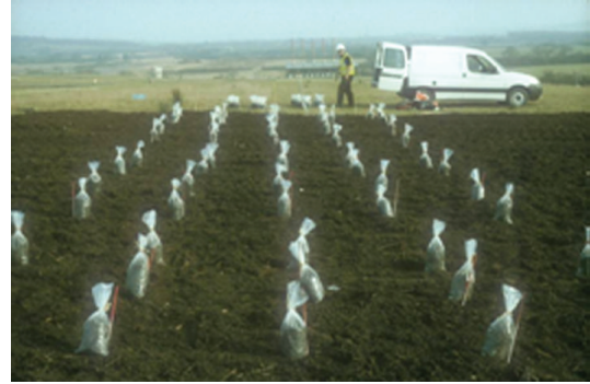
FIGURE 12: Two litre Earthworm Inoculation Units (EIUs) ready for inoculation into an organically-enriched landfill cap in the south of England.
