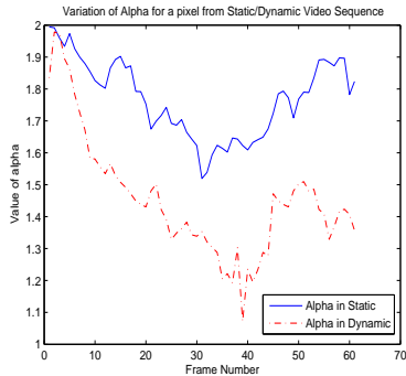
Fig. 6. (a) Estimated \alpha : in video from a static camera ( \alpha in static) and from a moving camera ( \alpha in dynamic)
