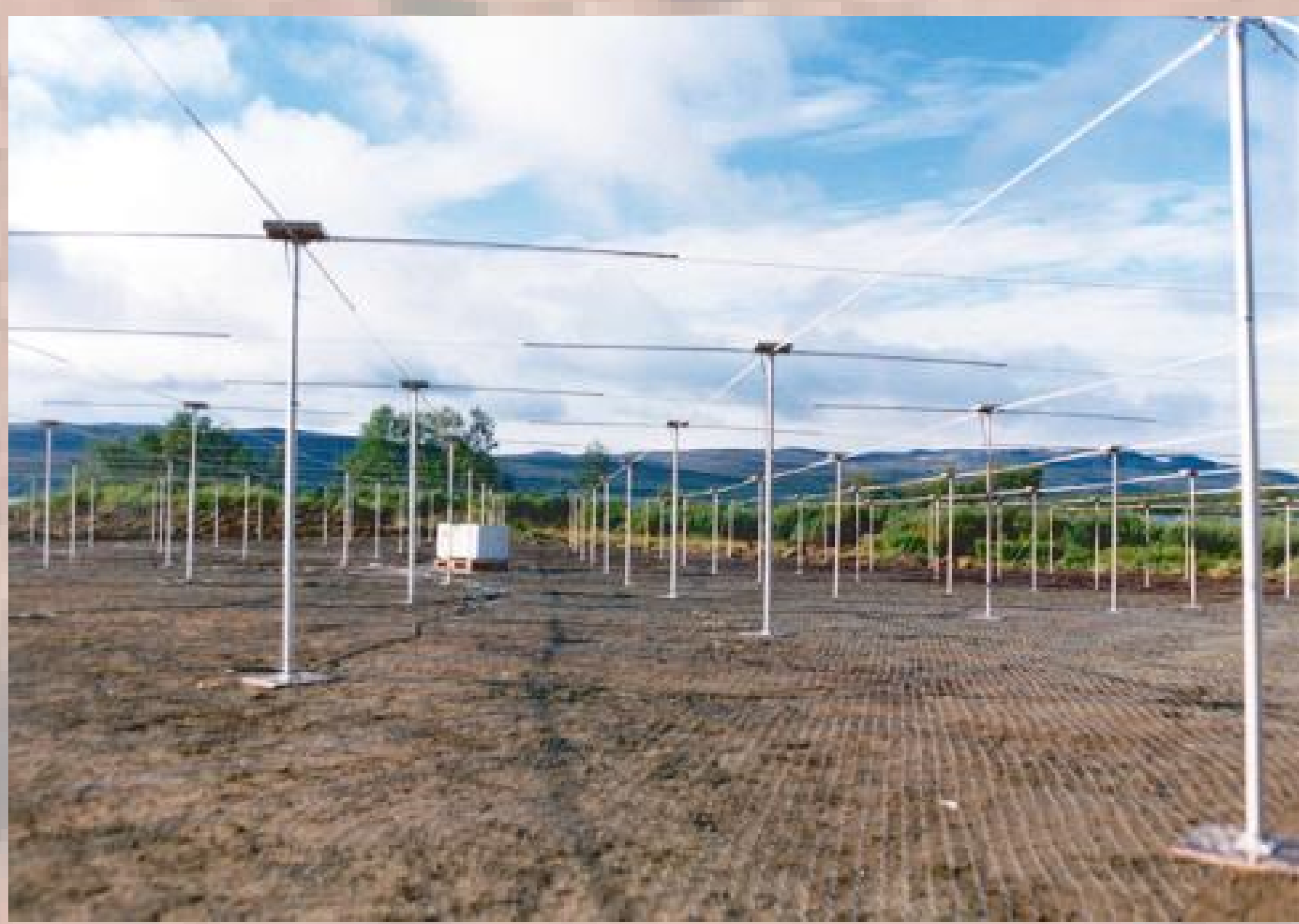
Ground-based imaging riometer system located in northern Finland.
