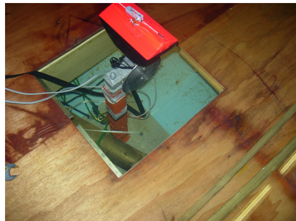
Fig. 3. Apparatus in tank – covers removed from seabed hatch to show pile.
