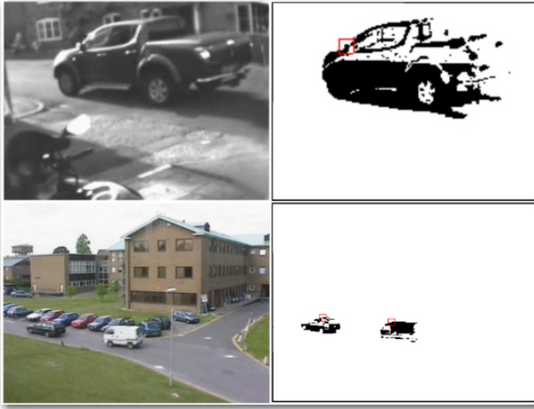
Fig. 5. Background Subtraction using the proposed RDE method, Left hand side scenes are original frames; right hand side scenes are modelled ones. The red square denotes the focal point of the foreground.
