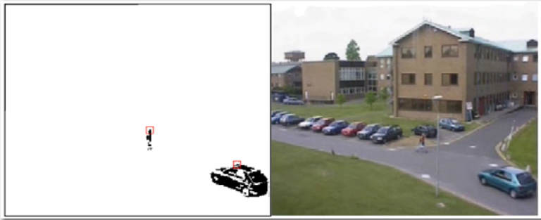
Fig. 4. Multi objects identification. Right hand side scenes are original frames; left hand side scenes are modelled ones. The red square denotes the focal point of the foreground.
