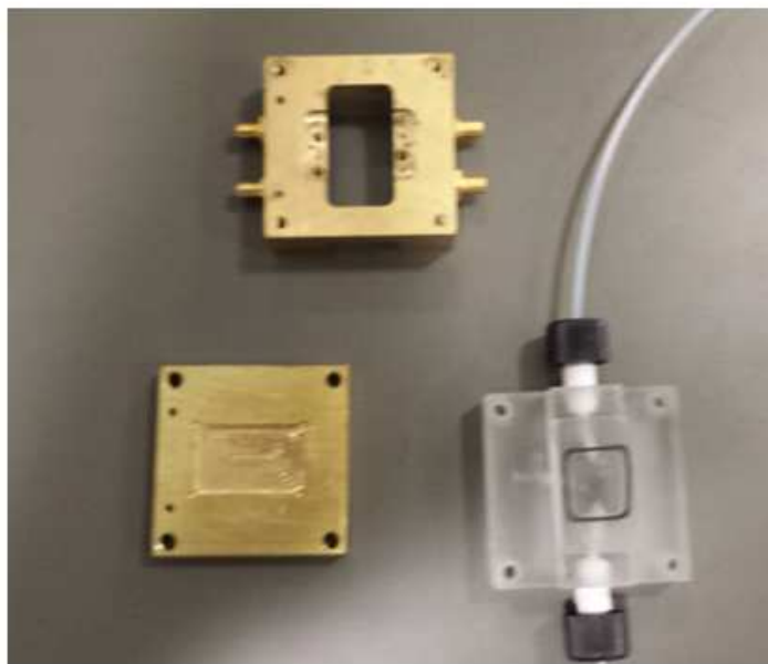
Figure 3.4: Parts of flow cell: bottom piece (bottom left), top piece (bottom right), middle piece (top)
