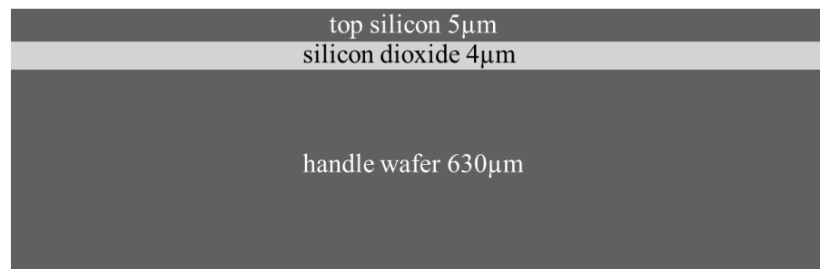
Fig. 3.3 Schematic illustration of SOI wafer for fabricating the suspended nanogap device
