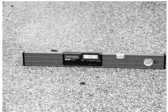
Figure 52. Digital level for measuring transverse and longitudinal grades.
