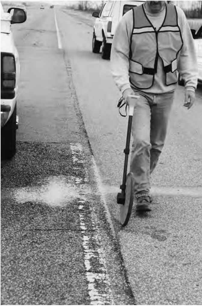
Figure 55. Measuring distances between core hole and drainage outlet.
