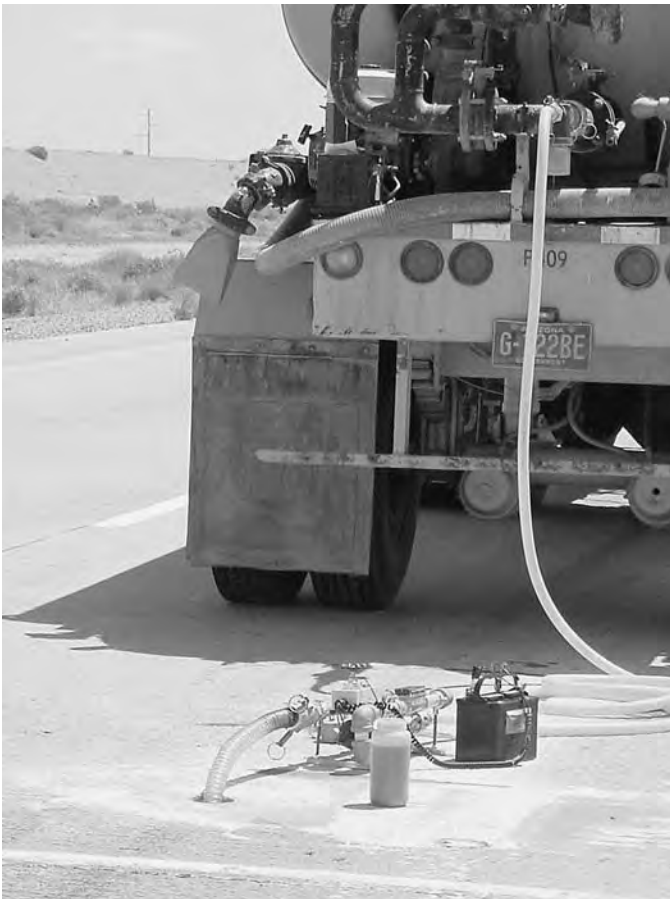
Figure 61. Water truck, connecting hose, flow meter, car battery, and tracer dye.
