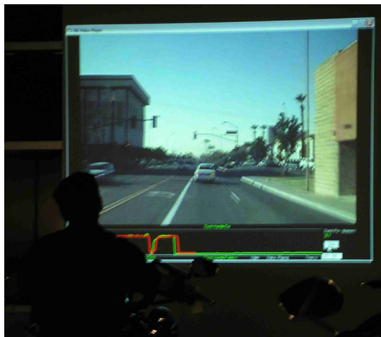
Figure 3: Participant following desired clutch profile by viewing his own clutch movement below simulation video.
