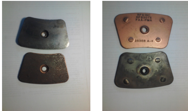
Figure 2.6: Oxidation of brake pad
