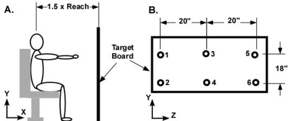
**Figure 2-1: Experimental Set-Up.** A. Sagittal view of the experimental set-up and B. frontal view of the target board with 6 LEDs arranged in 2 rows by 3 columns.
