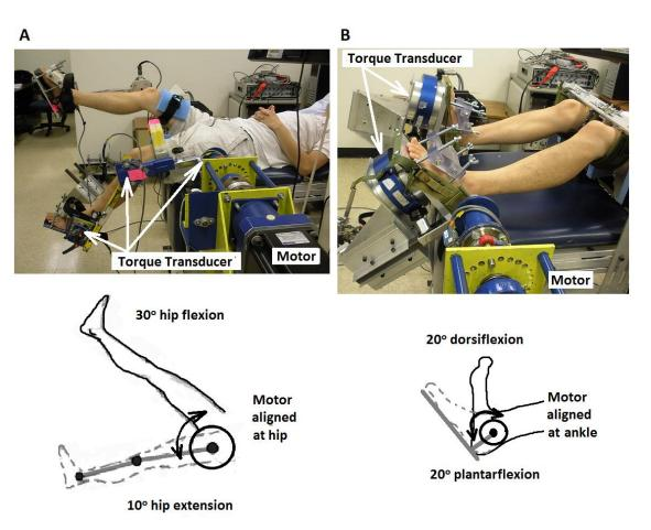
**Figure 2-1: Experimental Setup.** Leg robot used to impose bilateral hip oscillations and record sagittal plane torques during hip movements (A) and ankle movements (B). Two servomotor systems were used to impose movements about the hip and ankle joints. The hip joint was moved between  $30^{\circ}$  flexion and  $10^{\circ}$  extension, while the ankle joint was moved from  $20^{\circ}$  dorsiflexion to  $20^{\circ}$  plantarflexion.
