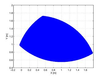
Figure 6.11: 3-R<u>P</u>R Reachable Workspace  $\phi = 0^{\circ}$
