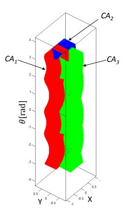
Figure 3.16: Only translational motion is possible due to the c-obstacles
