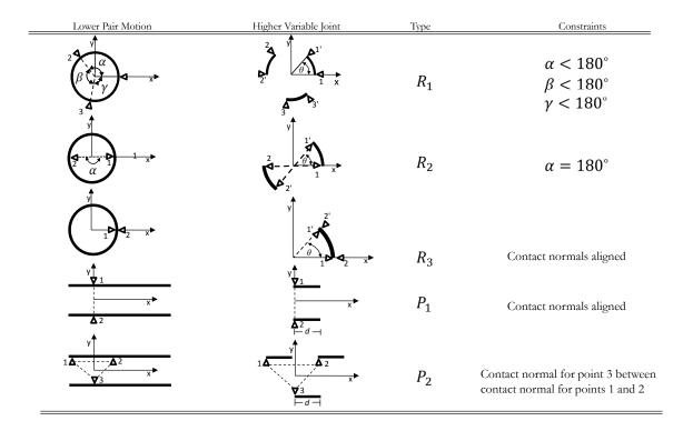
Figure 3.1: Higher Variable Joints
