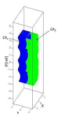
Figure 3.13: Only Translational Motion is Possible due to the C-obstacles
