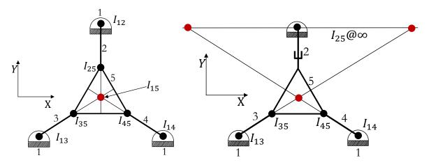
Figure 6.7: Singular Configuration
