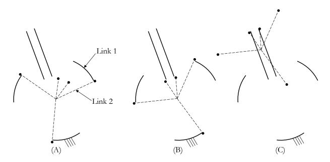
Figure 1.3: Rotational to Translational Variable Joint
