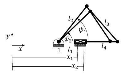
Figure 5.10: Two Position Rigid Body Guidance: RRRP
