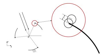
Figure 4.5: A Change of  $\delta_1$  in the Radial Direction
