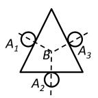
Figure 3.3: Rotation About the Z-axis is Possible
