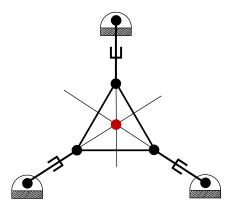
Figure 6.2: 3-RPR Singular Configuration
