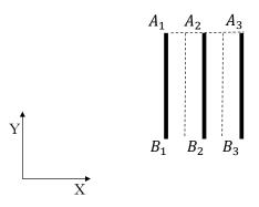
Figure 5.18: Three Position Rigid Body Guidance: RRRR
