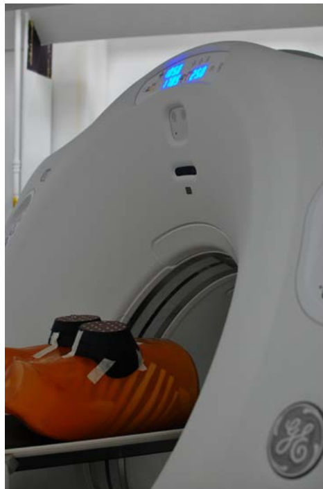
Figure 9. Lungman with RANDO phantom breast models attached and MOSFET dosimeters with leads.
