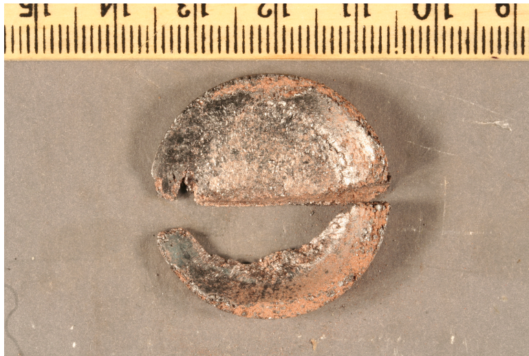
Figure H.4: Dynamically Compacted Powder at 0.34-0.433GPa Upon Removal from Gas Gun Target (Removed Cross Section for Imaging)
