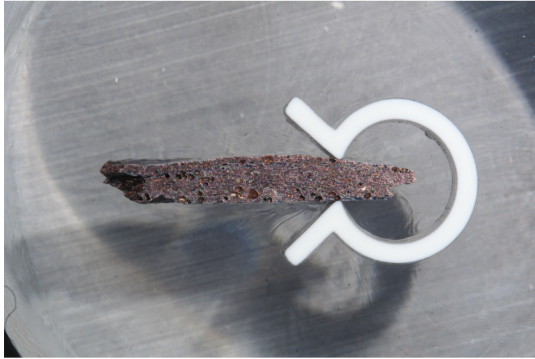
Figure H.3: Cross Section of Dynamically Compacted Powder at 0.34-0.433GPa.
