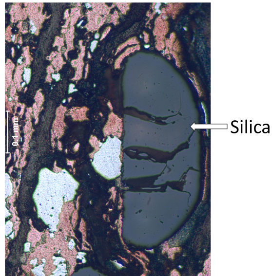
Figure 4.16: Optical Image of Dynamically Compacted Powder at 0.203GPa. Direction of Shock Wave is From the Left to Right
