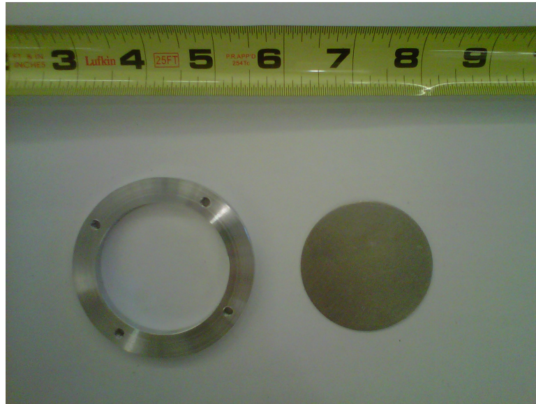
Figure F.3: Powder Container and Aluminum Back Piston
