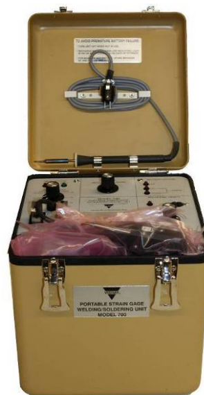
Figure 3.10 Vishay Spot Welder for Weldable Strain Gauges
