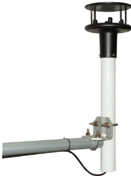
Figure 3.16 Gill Windsonic 2-D Sonic Anemometer (Gill 2010)
