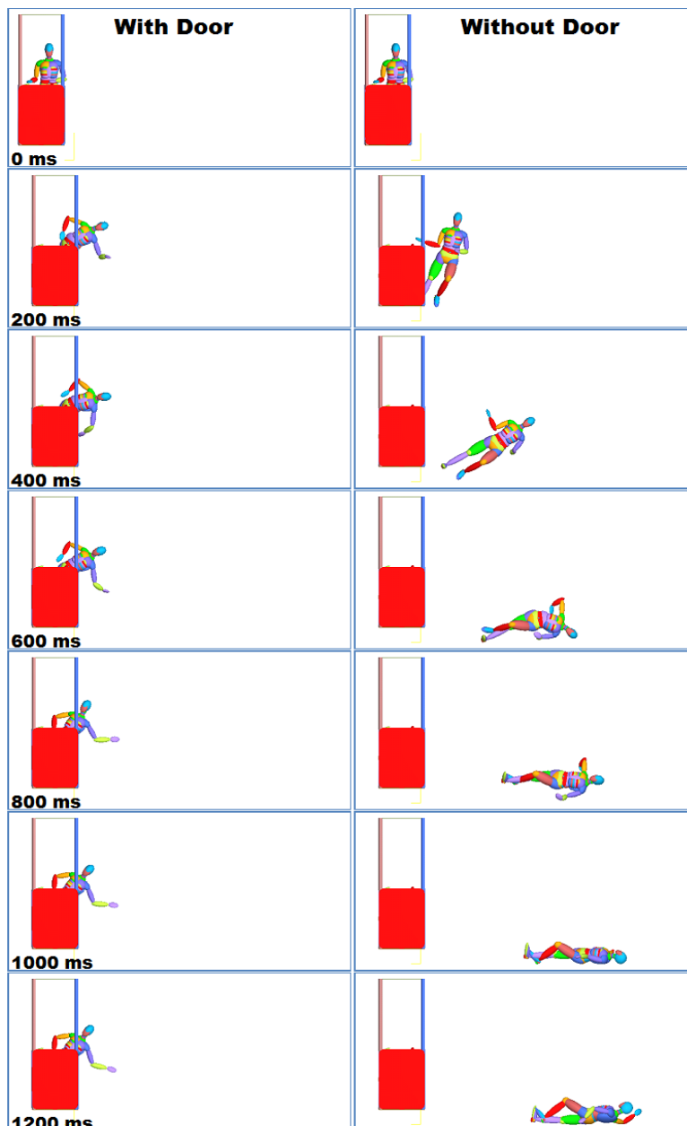
Figure 39: Fall progression comparison of door and no door trials for \Delta V of 16.1 km/h (10 mph) and no grip
