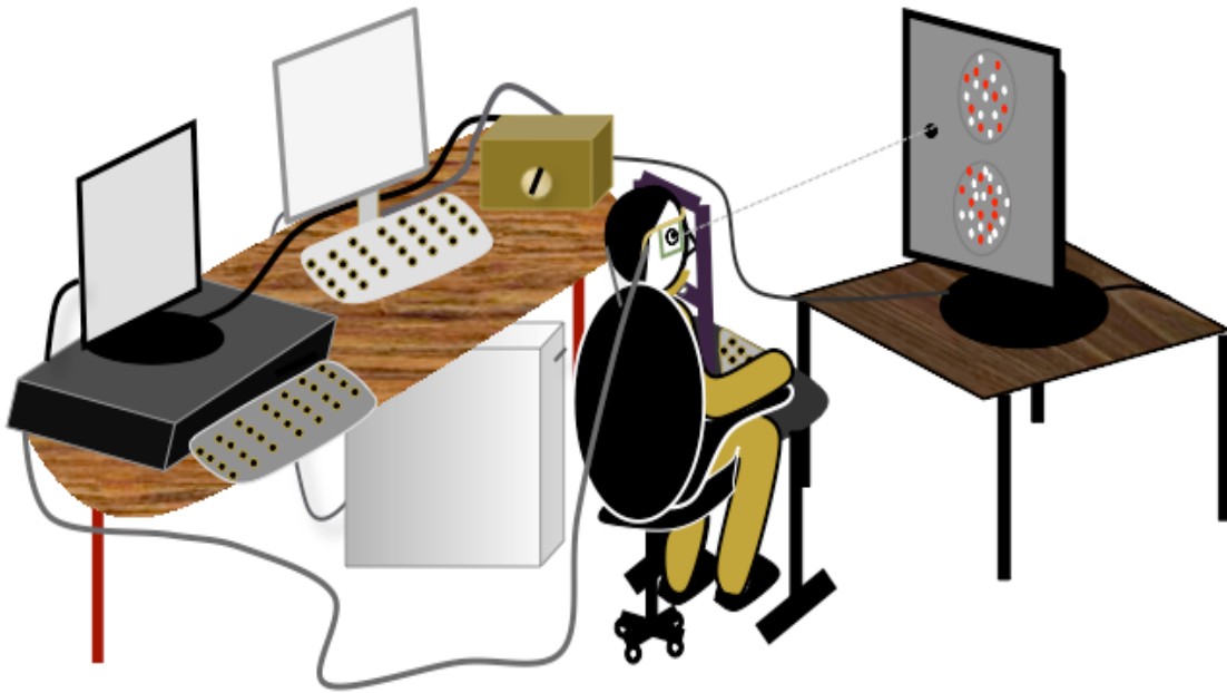
Figure 3-2. Experimental Setup. Fixation on the screen was presented either on the left or right side of screen to maximize the visual display of the stimulus and restrict the stimulus to a single visual field. The head and chin rest was used to hold the subjects head in a place while the experiment was conducted and the Eye tracker goggles were on at the same time to track the pupil movements of the eye.
