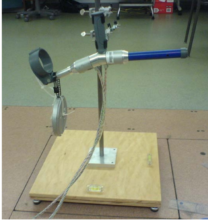
A.1.4.2. Two lbs load applied to the upper sensor in the Y-direction (ISB: X-direction)
