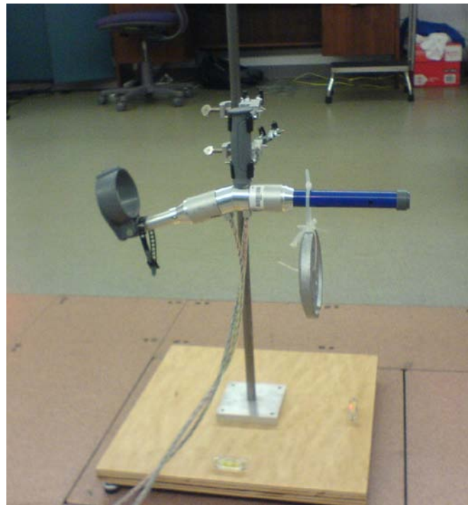
A.1.4.1 Two lb load applied to the lower sensor in the Y-direction (ISB: X-direction)
