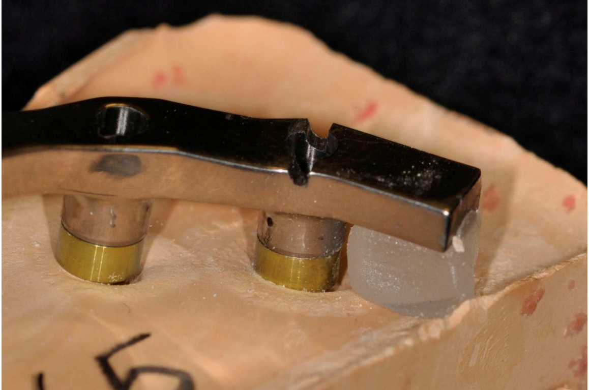
Figure 11: Light cured tray resin material between framework cantilever and stone model specimen to prevent downward movement of framework when measurements were done.
