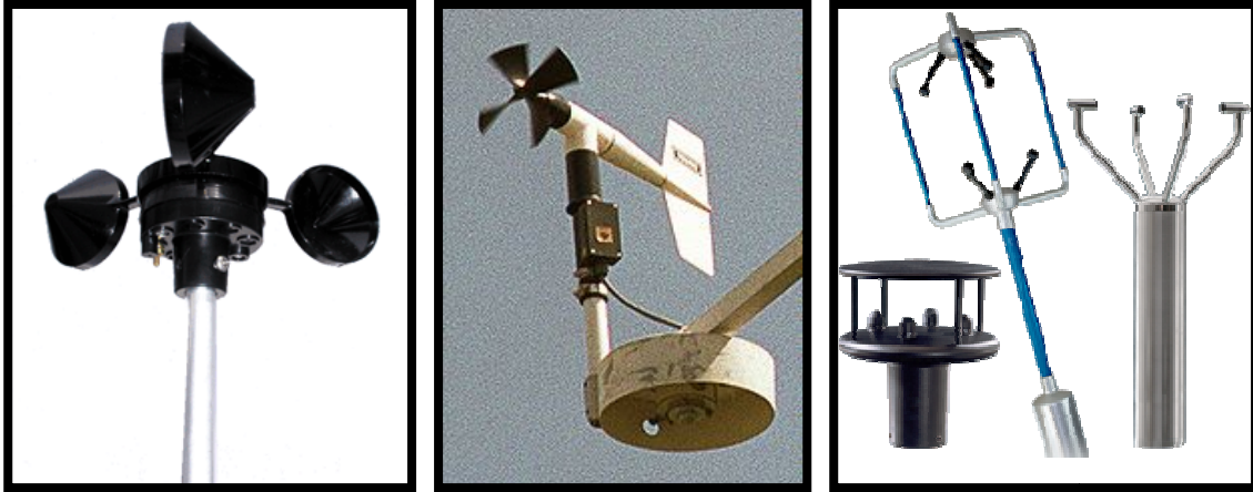
Figures 3.1.16, 3.1.17, 3.1.18: 3-Cup Anemometer, Windmill Anemometer, Sonic Anemometers 10
