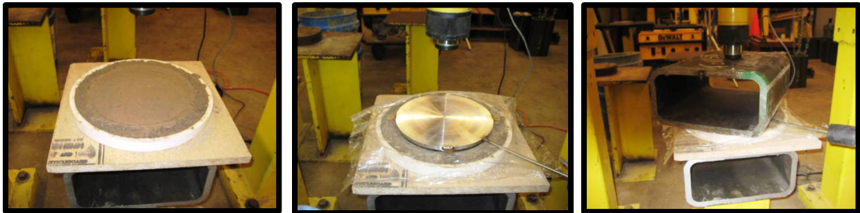
Figures 3.1.4, 3.1.5, and 3.1.6: Calibration Process for Spread Footing Earth Pressure Cell
