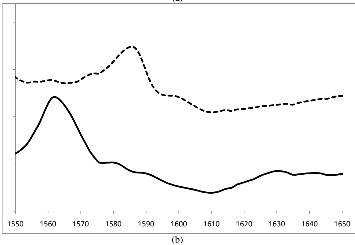
Figure 3-19. Infrared spectrum of free base porphyrone and iron porphyrone complexes in KBr powder: (a) 1000\text{ cm}^{-1} - 1250\text{ cm}^{-1} ; (b) 1550\text{ cm}^{-1} - 1650\text{ cm}^{-1} .
