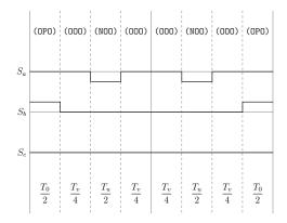
Figure A.53: Method 2 switching table Sector III, equivalent two-level sector V.
