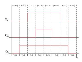
Figure 2.12: The division of the switching states in Sector V.
