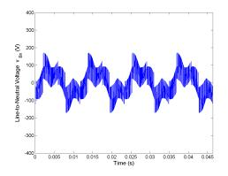
Figure 5.24: Line-to-neutral voltage  $v_{Bn}$  for Method 1 half rated speed, rated load.
