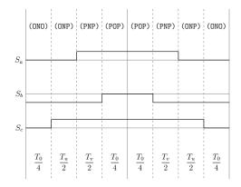
Figure A.35: Method 1 switching table Sector VI, equivalent two-level sector V.
