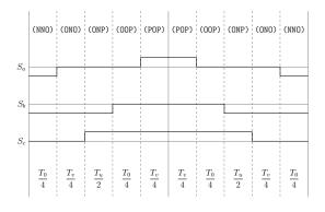
Figure A.102: Method 3 switching table Sector V, equivalent two-level sector VI.
