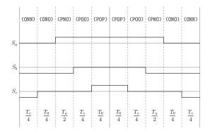
Figure A.103: Method 3 switching table Sector VI, equivalent two-level sector I.
