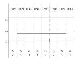
Figure A.72: Method 2 switching table Sector VI, equivalent two-level sector VI.
