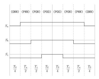
Figure A.1: Method 1 switching table Sector I, equivalent two-level sector I.
