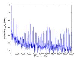
Figure 5.77: FFT of phase current  $i_A$  for Method 2 rated speed, rated load and  $C_{bus} = 400 mF$ .
