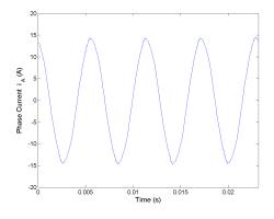
Figure 5.76: Phase current  $i_A$  for Method 2 rated speed, rated load and  $C_{bus} = 400 mF$ .
