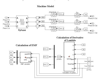
Figure 4.1: Circuit representation of the state space equations for the given IPM machine.
