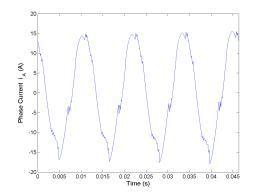
Figure 5.97: Phase current  $i_A$  for Method 2 half rated speed, rated load.
