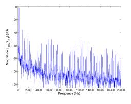
Figure 5.18: FFT of phase current  $i_C$  for Method 1 rated speed, rated load.
