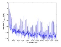
Figure 5.60: FFT of phase current  $i_C$  for Method 2 rated speed, rated load.
