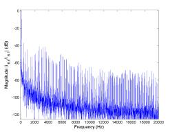
Figure 5.121: FFT of phase current  $i_B$  for Method 2 half rated speed, rated load and  $C_{bus} = 400 mF$ .
