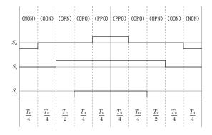
Figure A.85: Method 3 switching table Sector III, equivalent two-level sector I.
