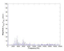
Figure 5.115: FFT of line-to-line voltage  $v_{BC}$  for Method 2 half rated speed, rated load and  $C_{bus} = 400 mF$ .
