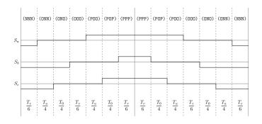
Figure A.104: Method 3 switching table Sector VI, equivalent two-level sector II.
