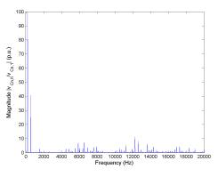
Figure 5.6: FFT of line-to-neutral voltage  $v_{Cn}$  for Method 1 rated speed, rated load.
