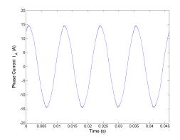
Figure 5.34: Phase current  $i_A$  for Method 1 half rated speed, rated load.
