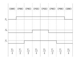
Figure A.6: Method 1 switching table Sector I, equivalent two-level sector VI.
