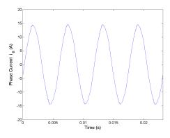
Figure 5.78: Phase current  $i_B$  for Method 2 rated speed, rated load and  $C_{bus} = 400 m F.$
