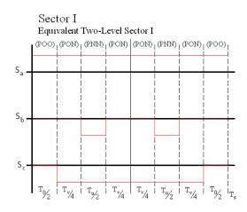
Figure 3.12: Method 2 switching pattern in Sector I, two-level sector I.
