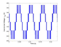
Figure 5.70: Line-to-line voltage  $v_{AB}$  for Method 2 rated speed, rated load and  $C_{bus} = 400 m F$ .
