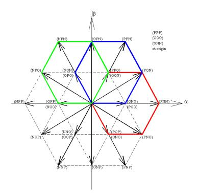
Figure 3.5: Two-level hexagons within the three-level hexagon. that sector. In Figure 3.7, the hexagon corresponding to sector I is shown.
