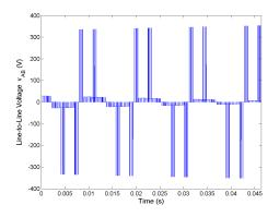
Figure 5.91: Line-to-line voltage  $v_{AB}$  for Method 2 half rated speed, rated load.
