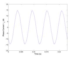
Figure 5.80: Phase current  $i_C$  for Method 2 rated speed, rated load and  $C_{bus} = 400 m F.$
