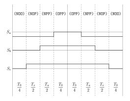
Figure A.22: Method 1 switching table Sector IV, equivalent two-level sector IV.
