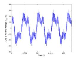
Figure 5.127: Line-to-neutral voltage  $v_{An}$  for Method 3 rated speed, rated load.
