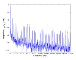
Figure 5.16: FFT of phase current  $i_B$  for Method 1 rated speed, rated load.
