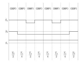
Figure A.65: Method 2 switching table Sector V, equivalent two-level sector V.
