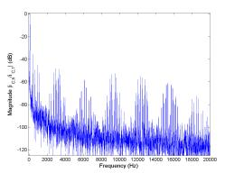
Figure 5.165: FFT of phase current  $i_C$  for Method 3 half rated speed, rated load.
