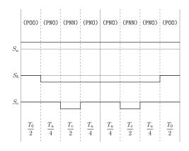
Figure A.42: Method 2 switching table Sector I, equivalent two-level sector VI.
