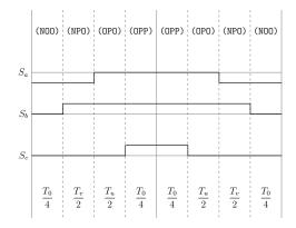
Figure A.20: Method 1 switching table Sector IV, equivalent two-level sector II.
