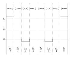
Figure A.39: Method 2 switching table Sector I, equivalent two-level sector III.
