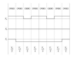
Figure A.38: Method 2 switching table Sector I, equivalent two-level sector II.
