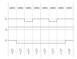
Figure A.50: Method 2 switching table Sector III, equivalent two-level sector II.
