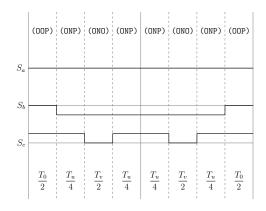
Figure A.66: Method 2 switching table Sector V, equivalent two-level sector VI.
