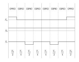
Figure A.45: Method 2 switching table Sector II, equivalent two-level sector III.
