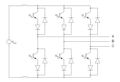
Figure 2.3: Basic two-level current source inverter.
