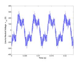
Figure 5.5: Line-to-neutral voltage  $v_{Cn}$  for Method 1 rated speed, rated load.
