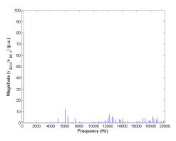
Figure 5.73: FFT of line-to-line voltage  $v_{BC}$  for Method 2 rated speed, rated load and  $C_{bus} = 400 mF$ .
