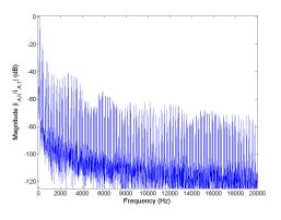
Figure 5.98: FFT of phase current  $i_A$  for Method 2 half rated speed, rated load.
