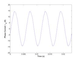
Figure 5.15: Phase current  $i_B$  for Method 1 rated speed, rated load.
