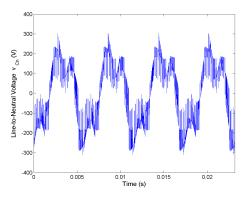
Figure 5.47: Line-to-neutral voltage  $v_{Cn}$  for Method 2 rated speed, rated load.
