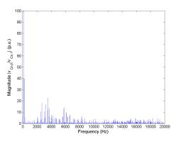
Figure 5.111: FFT of line-to-neutral voltage  $v_{Cn}$  for Method 2 half rated speed, rated load and  $C_{bus} = 400 mF$ .
