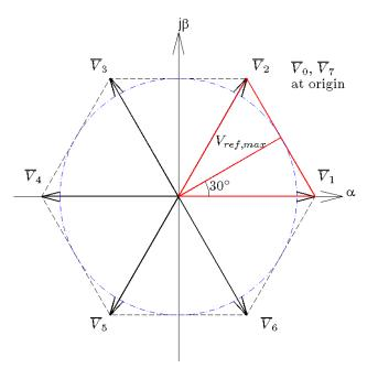
Figure 2.7: The maximum reference vector magnitude for linear modulation in the  $(\alpha - \beta)$  plane.
