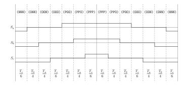
Figure A.75: Method 3 switching table Sector I, equivalent two-level sector III.
