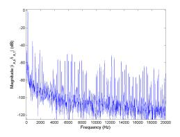
Figure 5.14: FFT of phase current  $i_A$  for Method 1 rated speed, rated load.
