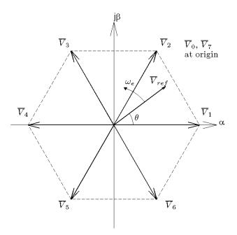
Figure 2.6: The reference space vector with the voltage vectors in the  $(\alpha - \beta)$  plane.
