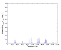
Figure 5.33: FFT of line-to-line voltage  $v_{CA}$  for Method 1 half rated speed, rated load.
