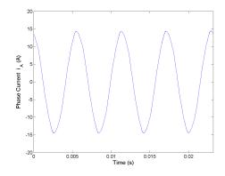
Figure 5.13: Phase current  $i_A$  for Method 1 rated speed, rated load.
