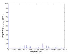
Figure 5.12: FFT of line-to-line voltage  $v_{CA}$  for Method 1 rated speed, rated load.
