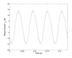
Figure 5.59: Phase current  $i_C$  for Method 2 rated speed, rated load.
