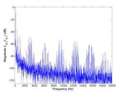
Figure 5.37: FFT of phase current  $i_B$  for Method 1 half rated speed, rated load.
