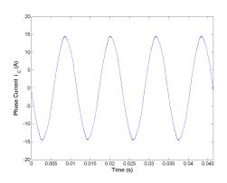
Figure 5.38: Phase current  $i_C$  for Method 1 half rated speed, rated load.
