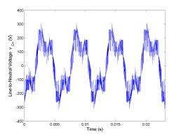
Figure 5.68: Line-to-neutral voltage  $v_{Cn}$  for Method 2 rated speed, rated load and  $C_{bus} = 400 mF$ .
