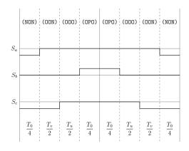
Figure A.18: Method 1 switching table Sector III, equivalent two-level sector VI.
