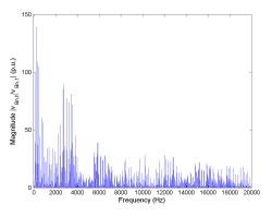
Figure 5.88: FFT of line-to-neutral voltage  $v_{Bn}$  for Method 2 half rated speed, rated load.
