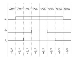
Figure A.108: Method 3 switching table Sector VI, equivalent two-level sector VI.
