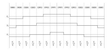
Figure A.82: Method 3 switching table Sector II, equivalent two-level sector IV.
