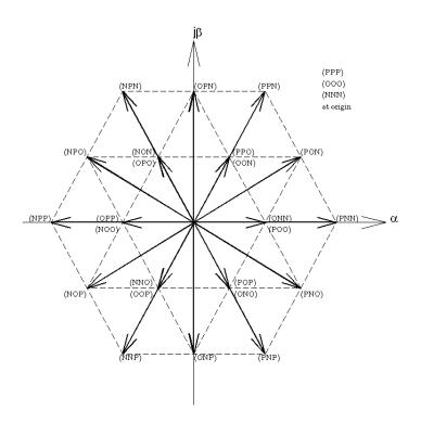
Figure 3.4: The three-level voltage vectors plotted in the  $(\alpha - \beta)$  plane.
