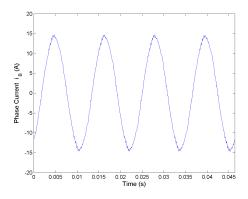
Figure 5.120: Phase current  $i_B$  for Method 2 half rated speed, rated load and  $C_{bus} = 400 mF$ .
