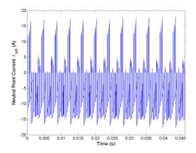
Figure 5.105: Neutral point current  $i_{NP}$  for Method 2 half rated speed, rated load. results are provided in the remainder of this section.
