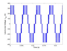
Figure 5.72: Line-to-line voltage  $v_{BC}$  for Method 2 rated speed, rated load and  $C_{bus} = 400 mF$ .
