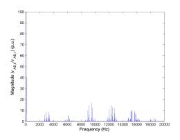
Figure 5.29: FFT of line-to-line voltage  $v_{AB}$  for Method 1 half rated speed, rated load.
