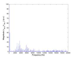
Figure 5.109: FFT of line-to-neutral voltage  $v_{Bn}$  for Method 2 half rated speed, rated load and  $C_{bus} = 400mF$ .
