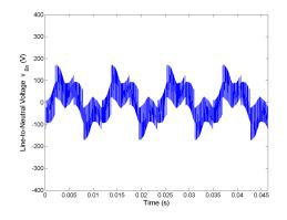
Figure 5.150: Line-to-neutral voltage  $v_{Bn}$  for Method 3 half rated speed, rated load.
