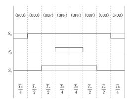
Figure A.24: Method 1 switching table Sector IV, equivalent two-level sector VI.
