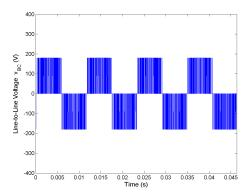
Figure 5.30: Line-to-line voltage  $v_{BC}$  for Method 1 half rated speed, rated load.
