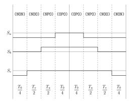
Figure A.16: Method 1 switching table Sector III, equivalent two-level sector IV.
