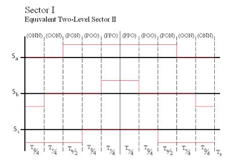
Figure 3.14: Method 3 switching pattern in Sector I, two-level sector II.
