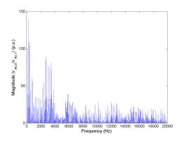
Figure 5.86: FFT of line-to-neutral voltage  $v_{An}$  for Method 2 half rated speed, rated load.
