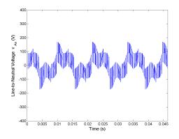
Figure 5.106: Line-to-neutral voltage  $v_{An}$  for Method 2 half rated speed, rated load and  $C_{bus} = 400 mF$ .
