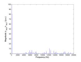
Figure 5.134: FFT of line-to-line voltage  $v_{AB}$  for Method 3 rated speed, rated load.
