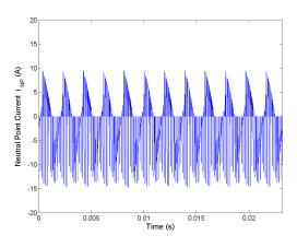
Figure 5.63: Neutral point current  $i_{NP}$  for Method 2 rated speed, rated load.
