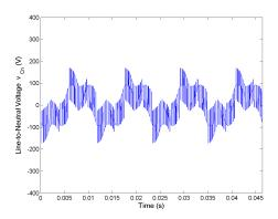
Figure 5.110: Line-to-neutral voltage  $v_{Cn}$  for Method 2 half rated speed, rated load and  $C_{bus} = 400 mF$ .
