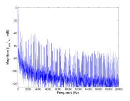
Figure 5.119: FFT of phase current  $i_A$  for Method 2 half rated speed, rated load and  $C_{bus} = 400 mF$ .
