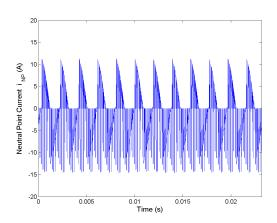
Figure 5.84: Neutral point current  $i_{NP}$  for Method 2 rated speed, rated load and  $C_{bus} = 400 mF$ .
