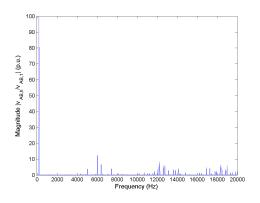
Figure 5.71: FFT of line-to-line voltage  $v_{AB}$  for Method 2 rated speed, rated load and  $C_{bus} = 400 mF$ .
