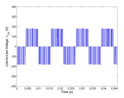
Figure 5.116: Line-to-line voltage  $v_{CA}$  for Method 2 half rated speed, rated load and  $C_{bus} = 400 mF$ .
