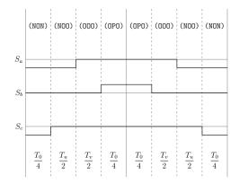
Figure A.17: Method 1 switching table Sector III, equivalent two-level sector V.
