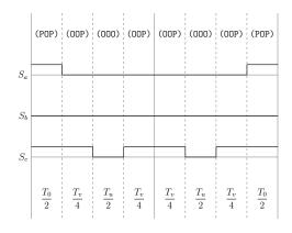
Figure A.69: Method 2 switching table Sector VI, equivalent two-level sector III.
