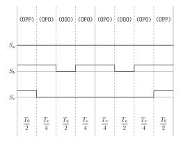
Figure A.55: Method 2 switching table Sector IV, equivalent two-level sector I.
