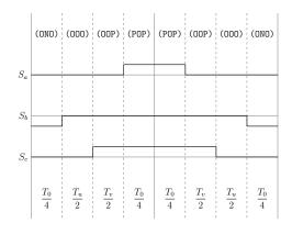
Figure A.33: Method 1 switching table Sector VI, equivalent two-level sector III.
