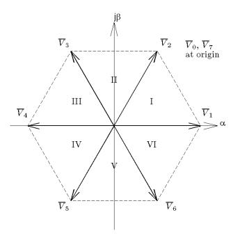
Figure 2.5: The voltage vectors plotted in the  $(\alpha - \beta)$  plane.
