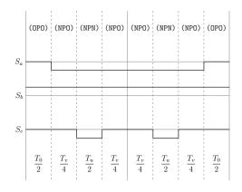
Figure A.51: Method 2 switching table Sector III, equivalent two-level sector III.
