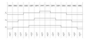
Figure A.98: Method 3 switching table Sector V, equivalent two-level sector II.
