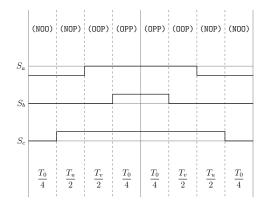
Figure A.23: Method 1 switching table Sector IV, equivalent two-level sector V.
