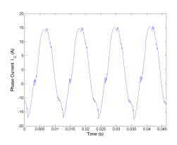
Figure 5.101: Phase current  $i_C$  for Method 2 half rated speed, rated load.
