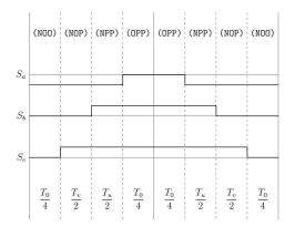
Figure A.94: Method 3 switching table Sector IV, equivalent two-level sector IV.
