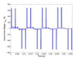
Figure 5.93: Line-to-line voltage  $v_{BC}$  for Method 2 half rated speed, rated load.
