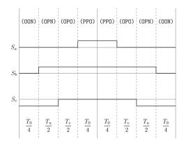
Figure A.9: Method 1 switching table Sector II, equivalent two-level sector III.
