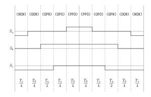
Figure A.81: Method 3 switching table Sector II, equivalent two-level sector III.
