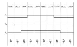
Figure A.95: Method 3 switching table Sector IV, equivalent two-level sector V.
