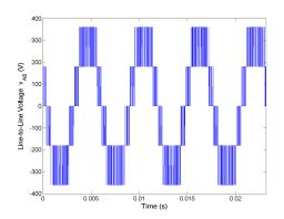
Figure 5.7: Line-to-line voltage  $v_{AB}$  for Method 1 rated speed, rated load.
