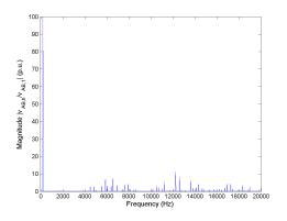
Figure 5.8: FFT of line-to-line voltage  $v_{AB}$  for Method 1 rated speed, rated load.
