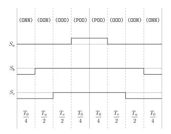
Figure A.3: Method 1 switching table Sector I, equivalent two-level sector III.
