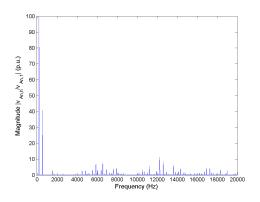
Figure 5.128: FFT of line-to-neutral voltage  $v_{An}$  for Method 3 rated speed, rated load.
