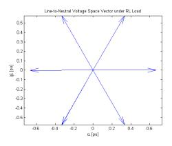
Figure 2.17: Space vector representation of the line-to-neutral voltage in the  $(\alpha - \beta)$  plane.
