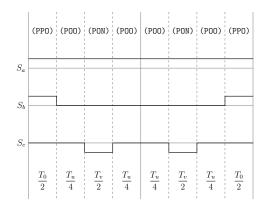
Figure A.48: Method 2 switching table Sector II, equivalent two-level sector VI.
