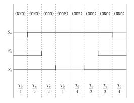
Figure A.25: Method 1 switching table Sector V, equivalent two-level sector I.
