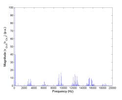
Figure 5.153: FFT of line-to-neutral voltage  $v_{Cn}$  for Method 3 half rated speed, rated load.
