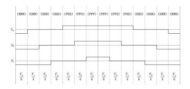
Figure A.83: Method 3 switching table Sector II, equivalent two-level sector V.
