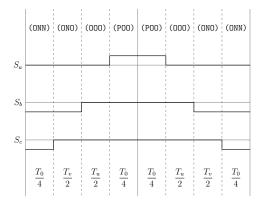
Figure A.4: Method 1 switching table Sector I, equivalent two-level sector IV.
