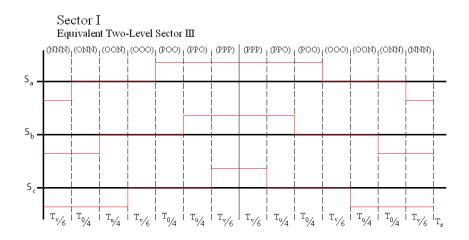
Figure 3.15: Method 3 switching pattern in Sector I, two-level sector III.
