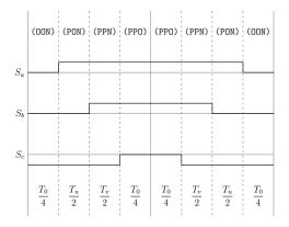
Figure A.7: Method 1 switching table Sector II, equivalent two-level sector I.
