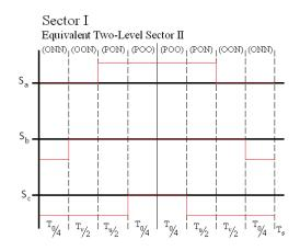
Figure 3.10: Method 1 switching pattern in Sector I, two-level sector I.
