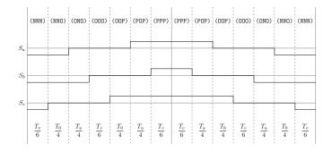
Figure A.97: Method 3 switching table Sector V, equivalent two-level sector I.
