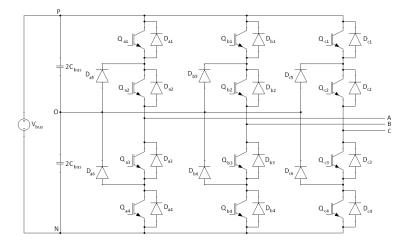
Figure 3.1: Three-level neutral-point-clamped inverter.
