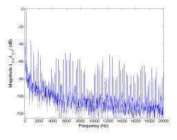
Figure 5.144: FFT of phase current  $i_C$  for Method 3 rated speed, rated load.
