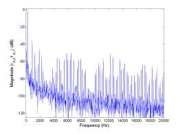
Figure 5.140: FFT of phase current  $i_A$  for Method 3 rated speed, rated load.
