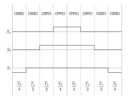
Figure A.10: Method 1 switching table Sector II, equivalent two-level sector IV.
