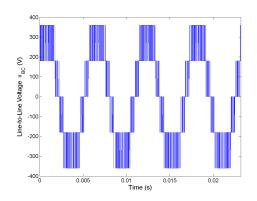
Figure 5.9: Line-to-line voltage  $v_{BC}$  for Method 1 rated speed, rated load.
