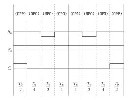
Figure A.56: Method 2 switching table Sector IV, equivalent two-level sector II.
