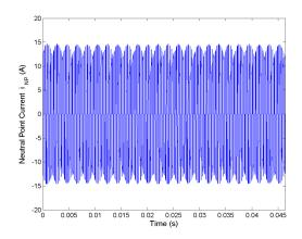
Figure 5.42: Neutral point current  $i_{NP}$  for Method 1 half rated speed, rated load.
