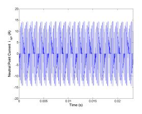
Figure 5.21: Neutral point current  $i_{NP}$  for Method 1 rated speed, rated load.
