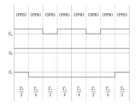
Figure A.44: Method 2 switching table Sector II, equivalent two-level sector II.
