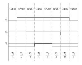
Figure A.73: Method 3 switching table Sector I, equivalent two-level sector I.
