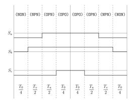
Figure A.86: Method 3 switching table Sector III, equivalent two-level sector II.
