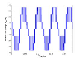
Figure 5.49: Line-to-line voltage  $v_{AB}$  for Method 2 rated speed, rated load.
