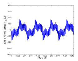
Figure 5.152: Line-to-neutral voltage  $v_{Cn}$  for Method 3 half rated speed, rated load.
