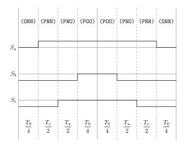
Figure A.78: Method 3 switching table Sector I, equivalent two-level sector VI.
