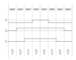
Figure A.93: Method 3 switching table Sector IV, equivalent two-level sector III.
