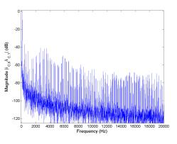
Figure 5.123: FFT of phase current  $i_C$  for Method 2 half rated speed, rated load and  $C_{bus} = 400 mF$ .
