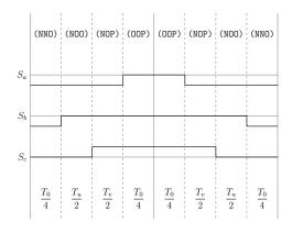
Figure A.27: Method 1 switching table Sector V, equivalent two-level sector III.
