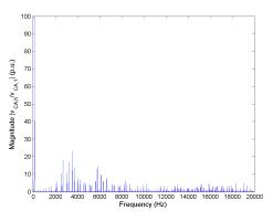
Figure 5.117: FFT of line-to-line voltage  $v_{CA}$  for Method 2 half rated speed, rated load and  $C_{bus} = 400 mF$ .
