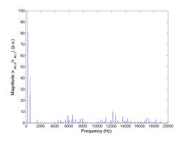
Figure 5.2: FFT of line-to-neutral voltage  $v_{An}$  for Method 1 rated speed, rated load.
