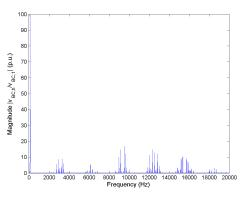
Figure 5.157: FFT of line-to-line voltage  $v_{BC}$  for Method 3 half rated speed, rated load.
