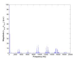
Figure 5.27: FFT of line-to-neutral voltage  $v_{Cn}$  for Method 1 half rated speed, rated load.
