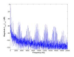
Figure 5.161: FFT of phase current  $i_A$  for Method 3 half rated speed, rated load.
