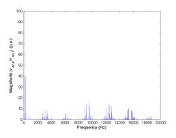
Figure 5.23: FFT of line-to-neutral voltage  $v_{An}$  for Method 1 half rated speed, rated load.
