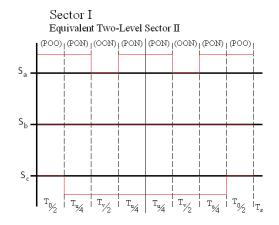
Figure 3.13: Method 2 switching pattern in Sector I, two-level sector II.
