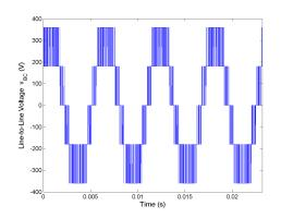
Figure 5.135: Line-to-line voltage  $v_{BC}$  for Method 3 rated speed, rated load.
