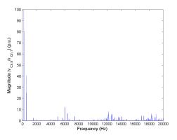
Figure 5.69: FFT of line-to-neutral voltage  $v_{Cn}$  for Method 2 rated speed, rated load and  $C_{bus} = 400 mF$ .
