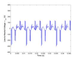
Figure 5.89: Line-to-neutral voltage  $v_{Cn}$  for Method 2 half rated speed, rated load.
