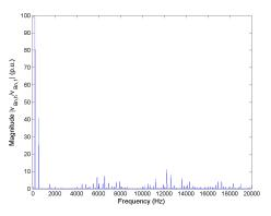
Figure 5.4: FFT of line-to-neutral voltage  $v_{Bn}$  for Method 1 rated speed, rated load.
