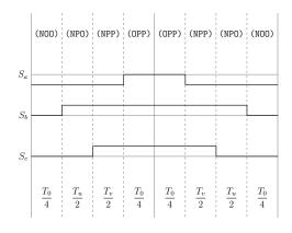
Figure A.21: Method 1 switching table Sector IV, equivalent two-level sector III.
