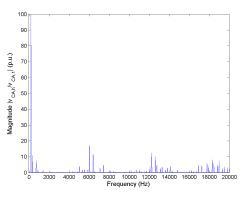
Figure 5.54: FFT of line-to-line voltage  $v_{CA}$  for Method 2 rated speed, rated load.
