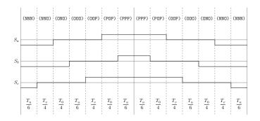
Figure A.105: Method 3 switching table Sector VI, equivalent two-level sector III.
