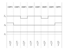
Figure A.59: Method 2 switching table Sector IV, equivalent two-level sector V.
