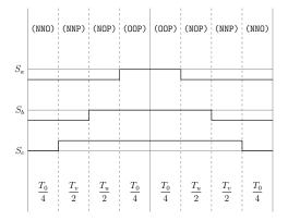
Figure A.100: Method 3 switching table Sector V, equivalent two-level sector IV.
