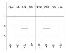
Figure A.37: Method 2 switching table Sector I, equivalent two-level sector I.
