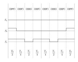
Figure A.60: Method 2 switching table Sector IV, equivalent two-level sector VI.
