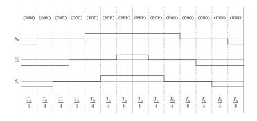
Figure A.76: Method 3 switching table Sector I, equivalent two-level sector IV.
