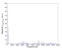
Figure 5.130: FFT of line-to-neutral voltage  $v_{Bn}$  for Method 3 rated speed, rated load.
