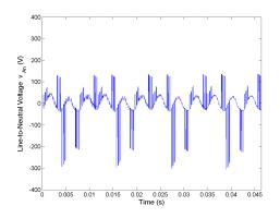
Figure 5.85: Line-to-neutral voltage  $v_{An}$  for Method 2 half rated speed, rated load.
