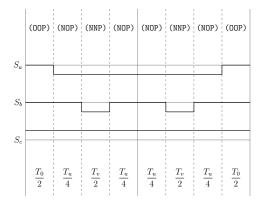
Figure A.64: Method 2 switching table Sector V, equivalent two-level sector IV.
