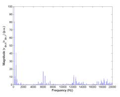
Figure 5.46: FFT of line-to-neutral voltage  $v_{Bn}$  for Method 2 rated speed, rated load.
