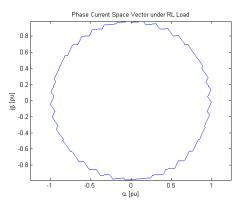
Figure 2.18: Space vector representation of the phase current in the  $(\alpha - \beta)$  plane.
