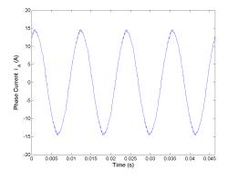
Figure 5.118: Phase current  $i_A$  for Method 2 half rated speed, rated load and  $C_{bus} = 400 mF$ .
