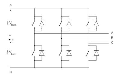
Figure 2.1: Generic two-level, three-phase inverter.
