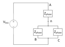
Figure 2.4: The equivalent load circuit for a switching state of  $S_1 = (1 \ 0 \ 0)$ .
