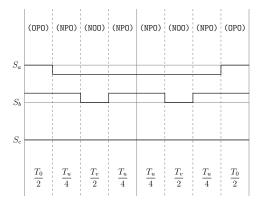
Figure A.52: Method 2 switching table Sector III, equivalent two-level sector IV.
