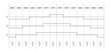
Figure A.96: Method 3 switching table Sector IV, equivalent two-level sector VI.
