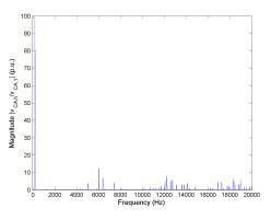
Figure 5.75: FFT of line-to-line voltage  $v_{CA}$  for Method 2 rated speed, rated load and  $C_{bus} = 400 mF$ .
