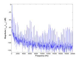
Figure 5.56: FFT of phase current  $i_A$  for Method 2 rated speed, rated load.
