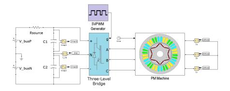
Figure 4.4: System model including inverter, space vector PWM generator, and PM machine.
