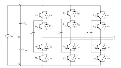
Figure 3.2: Three-level flying capacitor inverter.
