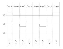
Figure A.40: Method 2 switching table Sector I, equivalent two-level sector IV.
