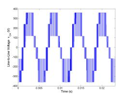
Figure 5.53: Line-to-line voltage  $v_{CA}$  for Method 2 rated speed, rated load.
