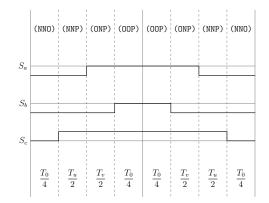
Figure A.101: Method 3 switching table Sector V, equivalent two-level sector V.
