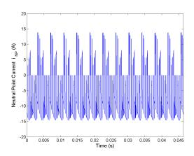
Figure 5.126: Neutral point current  $i_{NP}$  for Method 2 half rated speed, rated load and  $C_{bus} = 400 mF$ .
