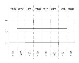
Figure A.87: Method 3 switching table Sector III, equivalent two-level sector III.
