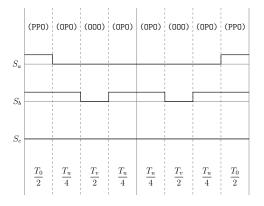
Figure A.46: Method 2 switching table Sector II, equivalent two-level sector IV.
