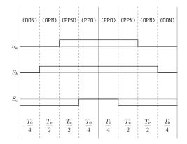
Figure A.80: Method 3 switching table Sector II, equivalent two-level sector II.
