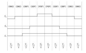
Figure A.106: Method 3 switching table Sector VI, equivalent two-level sector IV.
