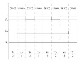
Figure A.41: Method 2 switching table Sector I, equivalent two-level sector V.
