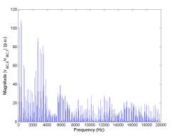
Figure 5.94: FFT of line-to-line voltage  $v_{BC}$  for Method 2 half rated speed, rated load.
