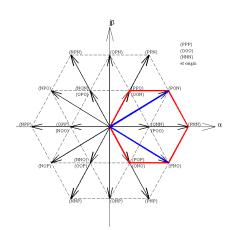
Figure 3.6: The division of the threelevel hexagon into sectors.
