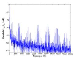
Figure 5.163: FFT of phase current  $i_B$  for Method 3 half rated speed, rated load.
