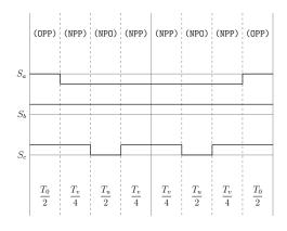
Figure A.57: Method 2 switching table Sector IV, equivalent two-level sector III.
