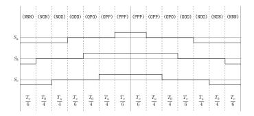
Figure A.89: Method 3 switching table Sector III, equivalent two-level sector V.
