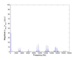
Figure 5.149: FFT of line-to-neutral voltage  $v_{An}$  for Method 3 half rated speed, rated load.
