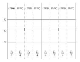
Figure A.49: Method 2 switching table Sector III, equivalent two-level sector I.
