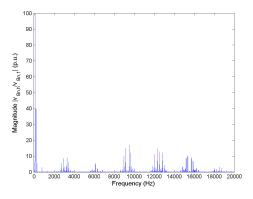
Figure 5.25: FFT of line-to-neutral voltage  $v_{Bn}$  for Method 1 half rated speed, rated load.
