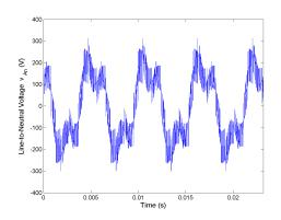
Figure 5.1: Line-to-neutral voltage  $v_{An}$  for Method 1 rated speed, rated load.
