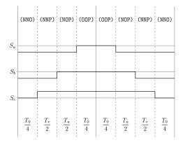
Figure A.28: Method 1 switching table Sector V, equivalent two-level sector IV.
