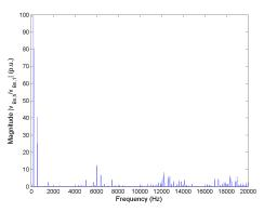
Figure 5.67: FFT of line-to-neutral voltage  $v_{Bn}$  for Method 2 rated speed, rated load and  $C_{bus} = 400 mF$ .
