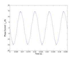
Figure 5.164: Phase current  $i_C$  for Method 3 half rated speed, rated load.
