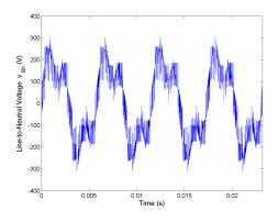
Figure 5.66: Line-to-neutral voltage  $v_{Bn}$  for Method 2 rated speed, rated load and  $C_{bus} = 400 mF$ .
