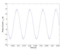
Figure 5.122: Phase current  $i_C$  for Method 2 half rated speed, rated load and  $C_{bus} = 400 mF$ .
