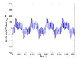
Figure 5.108: Line-to-neutral voltage  $v_{Bn}$  for Method 2 half rated speed, rated load and  $C_{bus} = 400 mF$ .
