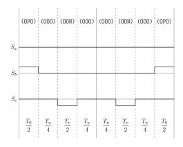
Figure A.54: Method 2 switching table Sector III, equivalent two-level sector VI.
