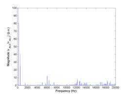
Figure 5.65: FFT of line-to-neutral voltage  $v_{An}$  for Method 2 rated speed, rated load and  $C_{bus} = 400 mF$ .
