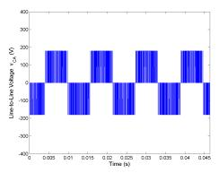
Figure 5.158: Line-to-line voltage  $v_{CA}$  for Method 3 half rated speed, rated load.
