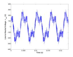
Figure 5.64: Line-to-neutral voltage  $v_{An}$  for Method 2 rated speed, rated load and  $C_{bus} = 400 mF$ .
