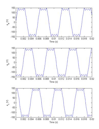
Figure 4.2: Simulated open circuit back emf of the IPM machine.
