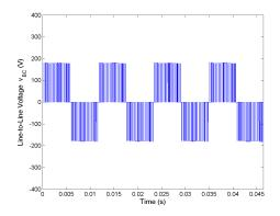
Figure 5.114: Line-to-line voltage  $v_{BC}$  for Method 2 half rated speed, rated load and  $C_{bus} = 400 mF$ .
