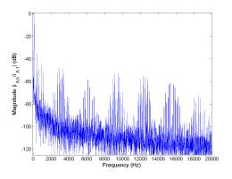
Figure 5.35: FFT of phase current  $i_A$  for Method 1 half rated speed, rated load.
