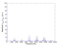
Figure 5.31: FFT of line-to-line voltage  $v_{BC}$  for Method 1 half rated speed, rated load.
