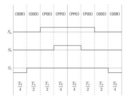
Figure A.11: Method 1 switching table Sector II, equivalent two-level sector V.
