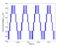
Figure 5.74: Line-to-line voltage  $v_{CA}$  for Method 2 rated speed, rated load and  $C_{bus} = 400 mF$ .
