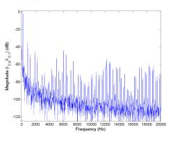
Figure 5.81: FFT of phase current  $i_C$  for Method 2 rated speed, rated load and  $C_{bus} = 400 mF$ .
