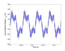
Figure 5.3: Line-to-neutral voltage  $v_{Bn}$  for Method 1 rated speed, rated load.
