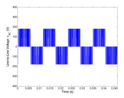
Figure 5.156: Line-to-line voltage  $v_{BC}$  for Method 3 half rated speed, rated load.
