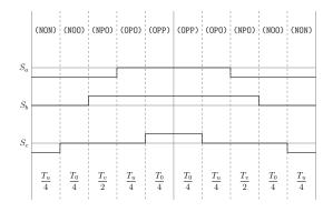
Figure A.92: Method 3 switching table Sector IV, equivalent two-level sector II.
