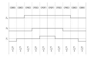
Figure A.77: Method 3 switching table Sector I, equivalent two-level sector V.
