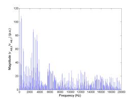
Figure 5.92: FFT of line-to-line voltage  $v_{AB}$  for Method 2 half rated speed, rated load.
