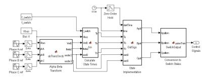
Figure 4.3: The generic space vector PWM pulse generator model.
