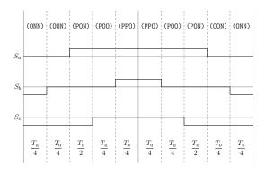
Figure A.84: Method 3 switching table Sector II, equivalent two-level sector VI.
