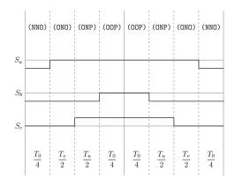
Figure A.30: Method 1 switching table Sector V, equivalent two-level sector VI.
