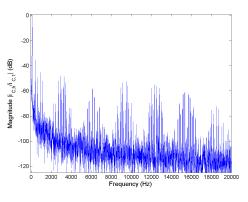
Figure 5.39: FFT of phase current  $i_C$  for Method 1 half rated speed, rated load.
