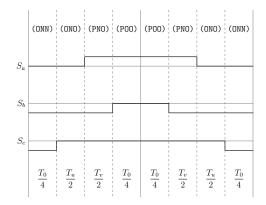
Figure A.5: Method 1 switching table Sector I, equivalent two-level sector V.
