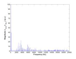
Figure 5.107: FFT of line-to-neutral voltage  $v_{An}$  for Method 2 half rated speed, rated load and  $C_{bus} = 400 mF$ .
