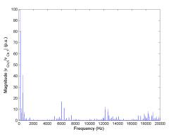
Figure 5.48: FFT of line-to-neutral voltage  $v_{Cn}$  for Method 2 rated speed, rated load.
