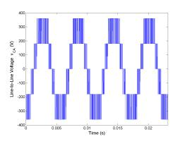
Figure 5.11: Line-to-line voltage  $v_{CA}$  for Method 1 rated speed, rated load.
