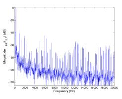
Figure 5.79: FFT of phase current  $i_B$  for Method 2 rated speed, rated load and  $C_{bus} = 400 mF$ .
