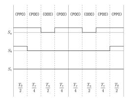
Figure A.47: Method 2 switching table Sector II, equivalent two-level sector V.
