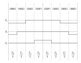
Figure A.26: Method 1 switching table Sector V, equivalent two-level sector II.
