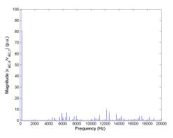
Figure 5.136: FFT of line-to-line voltage  $v_{BC}$  for Method 3 rated speed, rated load.
