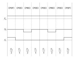
Figure A.67: Method 2 switching table Sector VI, equivalent two-level sector I.
