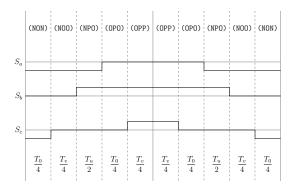
Figure A.88: Method 3 switching table Sector III, equivalent two-level sector IV.
