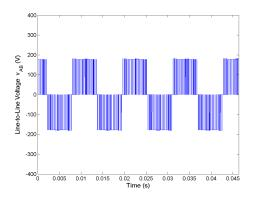
Figure 5.112: Line-to-line voltage  $v_{AB}$  for Method 2 half rated speed, rated load and  $C_{bus} = 400 mF$ .
