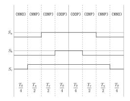
Figure A.29: Method 1 switching table Sector V, equivalent two-level sector V.
