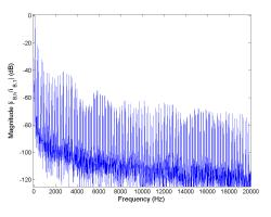
Figure 5.100: FFT of phase current  $i_B$  for Method 2 half rated speed, rated load.
