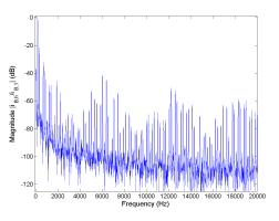
Figure 5.58: FFT of phase current  $i_B$  for Method 2 rated speed, rated load.
