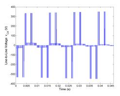
Figure 5.95: Line-to-line voltage  $v_{CA}$  for Method 2 half rated speed, rated load.
