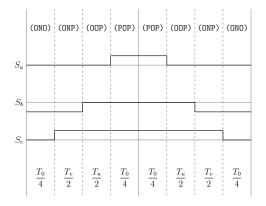
Figure A.34: Method 1 switching table Sector VI, equivalent two-level sector IV.
