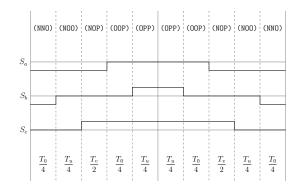
Figure A.99: Method 3 switching table Sector V, equivalent two-level sector III.
