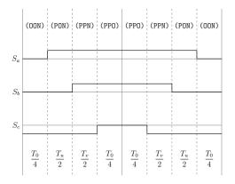
Figure A.79: Method 3 switching table Sector II, equivalent two-level sector I.
