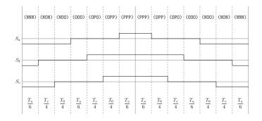
Figure A.91: Method 3 switching table Sector IV, equivalent two-level sector I.
