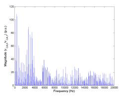
Figure 5.96: FFT of line-to-line voltage  $v_{CA}$  for Method 2 half rated speed, rated load.
