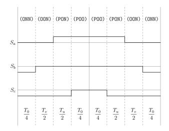
Figure A.2: Method 1 switching table Sector I, equivalent two-level sector II.
