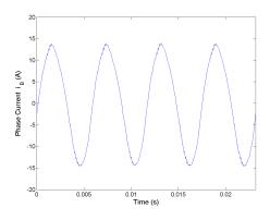
Figure 5.57: Phase current  $i_B$  for Method 2 rated speed, rated load.
