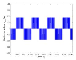
Figure 5.32: Line-to-line voltage  $v_{CA}$  for Method 1 half rated speed, rated load.
