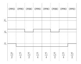
Figure A.43: Method 2 switching table Sector II, equivalent two-level sector I.
