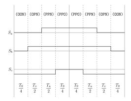
Figure A.8: Method 1 switching table Sector II, equivalent two-level sector II.
