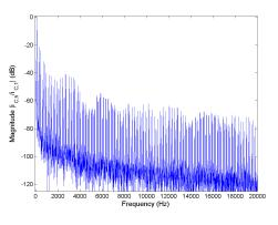
Figure 5.102: FFT of phase current  $i_C$  for Method 2 half rated speed, rated load.
