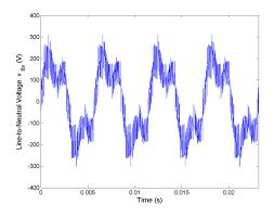
Figure 5.129: Line-to-neutral voltage  $v_{Bn}$  for Method 3 rated speed, rated load.
