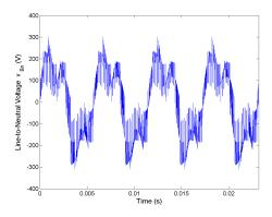
Figure 5.45: Line-to-neutral voltage  $v_{Bn}$  for Method 2 rated speed, rated load.
