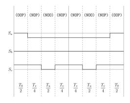
Figure A.63: Method 2 switching table Sector V, equivalent two-level sector III.
