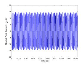
Figure 5.168: Neutral point current  $i_{NP}$  for Method 3 half rated speed, rated load.
