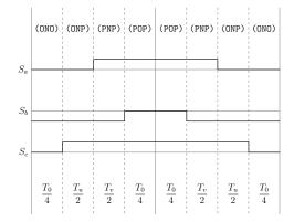
Figure A.107: Method 3 switching table Sector VI, equivalent two-level sector V.
