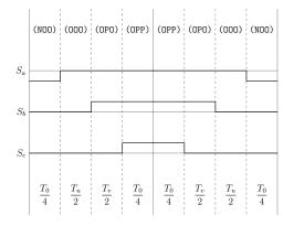
Figure A.19: Method 1 switching table Sector IV, equivalent two-level sector I.
