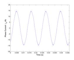
Figure 5.36: Phase current  $i_B$  for Method 1 half rated speed, rated load.
