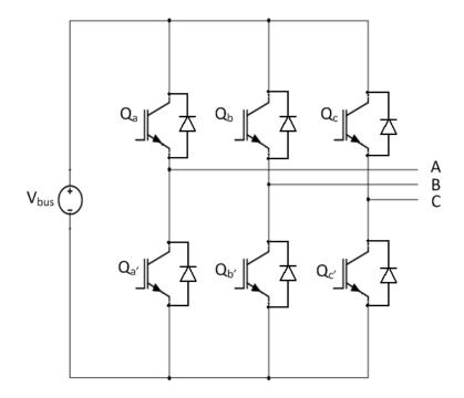
Figure 2.2: Basic two-level voltage source inverter.
