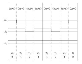
Figure A.58: Method 2 switching table Sector IV, equivalent two-level sector IV.
