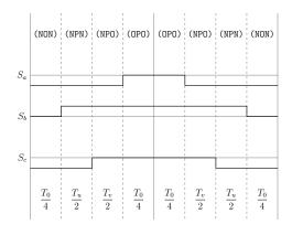
Figure A.15: Method 1 switching table Sector III, equivalent two-level sector III.
