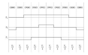
Figure A.74: Method 3 switching table Sector I, equivalent two-level sector II.
