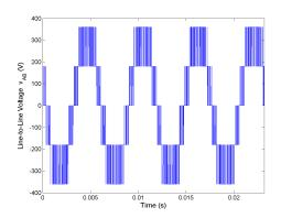
Figure 5.133: Line-to-line voltage  $v_{AB}$  for Method 3 rated speed, rated load.
