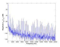
Figure 5.142: FFT of phase current  $i_B$  for Method 3 rated speed, rated load.
