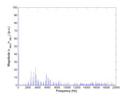
Figure 5.113: FFT of line-to-line voltage  $v_{AB}$  for Method 2 half rated speed, rated load and  $C_{bus} = 400 mF$ .
