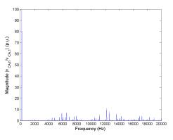
Figure 5.138: FFT of line-to-line voltage  $v_{CA}$  for Method 3 rated speed, rated load.
