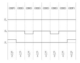
Figure A.61: Method 2 switching table Sector V, equivalent two-level sector I.
