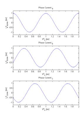
Figure 2.16: Time domain plot of the phase currents for an RL load using Two-Level SVM.
