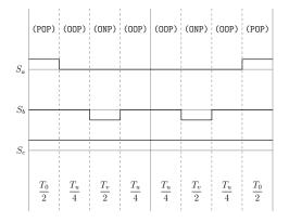
Figure A.70: Method 2 switching table Sector VI, equivalent two-level sector IV.
