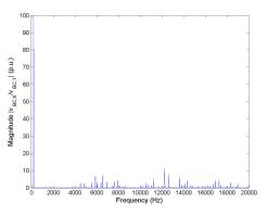
Figure 5.10: FFT of line-to-line voltage  $v_{BC}$  for Method 1 rated speed, rated load.
