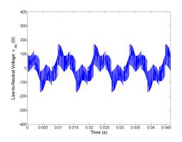
Figure 5.22: Line-to-neutral voltage  $v_{An}$  for Method 1 half rated speed, rated load.
