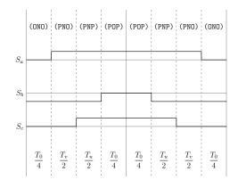
Figure A.36: Method 1 switching table Sector VI, equivalent two-level sector VI.
