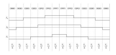
Figure A.90: Method 3 switching table Sector III, equivalent two-level sector VI.
