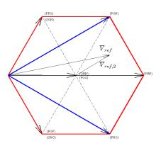
Figure 3.8: Mapping of the three-level voltage reference into the sector I two-level hexagon.
