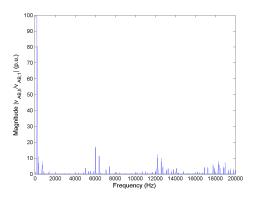
Figure 5.50: FFT of line-to-line voltage  $v_{AB}$  for Method 2 rated speed, rated load.
