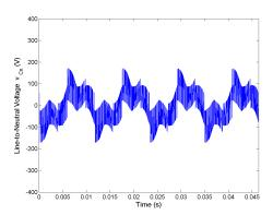
Figure 5.26: Line-to-neutral voltage  $v_{Cn}$  for Method 1 half rated speed, rated load.
