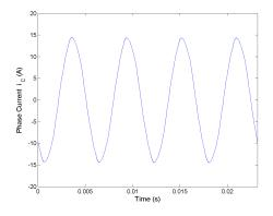
Figure 5.143: Phase current  $i_C$  for Method 3 rated speed, rated load.
