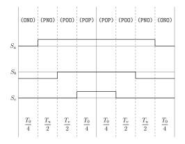
Figure A.31: Method 1 switching table Sector VI, equivalent two-level sector I.
