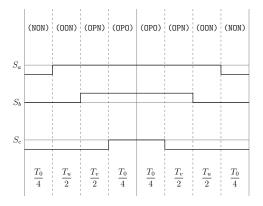
Figure A.13: Method 1 switching table Sector III, equivalent two-level sector I.
