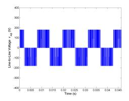
Figure 5.28: Line-to-line voltage  $v_{AB}$  for Method 1 half rated speed, rated load.
