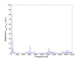
Figure 5.44: FFT of line-to-neutral voltage  $v_{An}$  for Method 2 rated speed, rated load.
