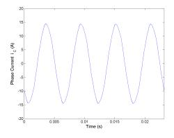
Figure 5.17: Phase current  $i_C$  for Method 1 rated speed, rated load.
