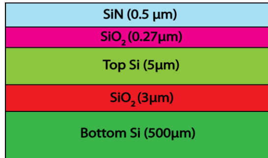
Figure 2-1-1. Wafer structure before fabrication.
