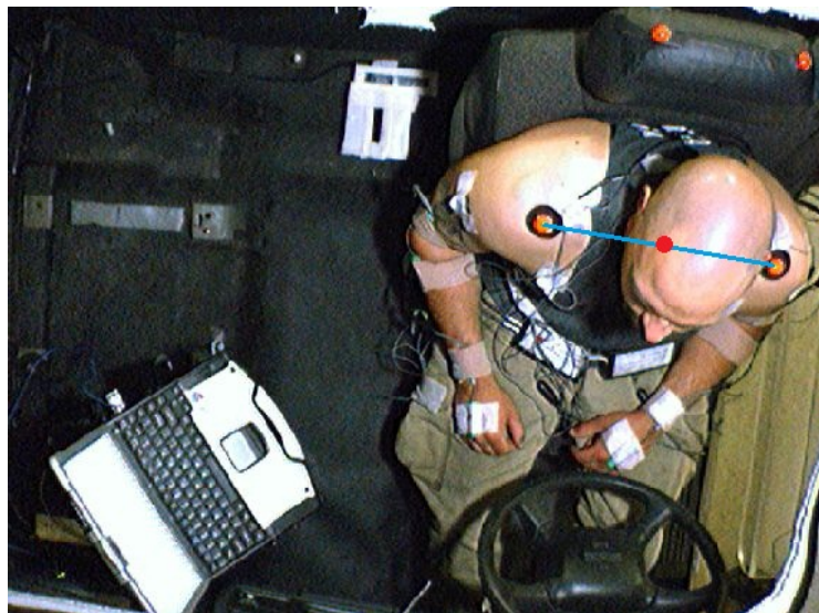
Figure 3.13. Middle of shoulders reference point (Red Dot) of a participant sitting relaxed against back of seat
