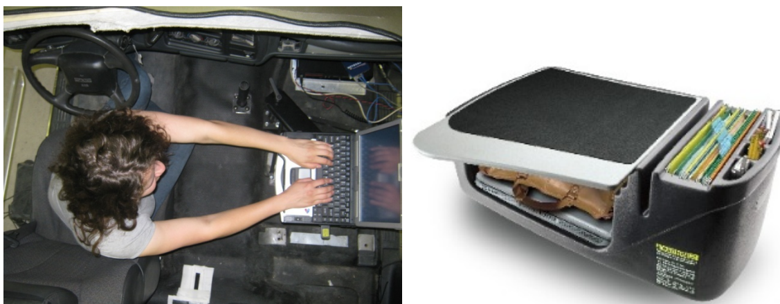
Figure 3.2. Location A - mobile computer mounted over passenger seat (Left) and passenger seat desk unit (Right)
