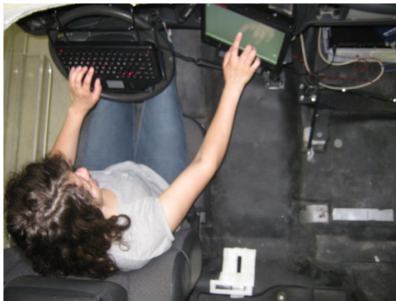
Figure 3.4. Location C - computer with display mounted on instrument panel and keyboard on steering wheel
