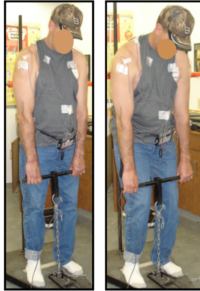
Figure 3.34. Maximal calibration apparatus setup for upper trapezius (Left) and erector spinae (Right)
