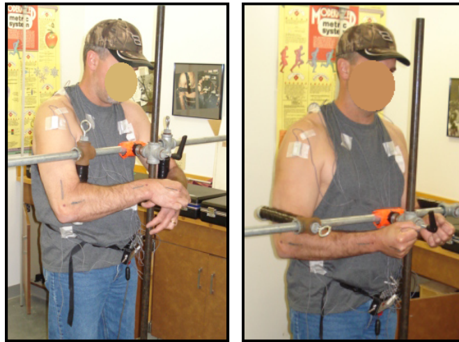
Figure 3.33. Maximal calibration apparatus setup for pectoralis major (Left) and middle deltoids (Right)
