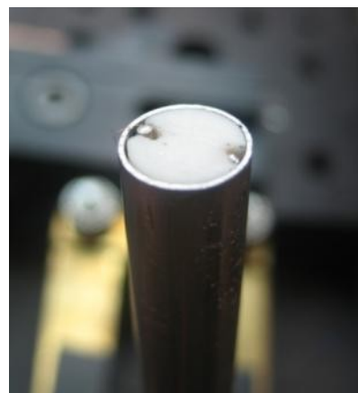
Fig. 2-21: Photo of the aluminum tubing slide over the side of the acrylic plug. The surface of the plug and tubing are flush with each other.
