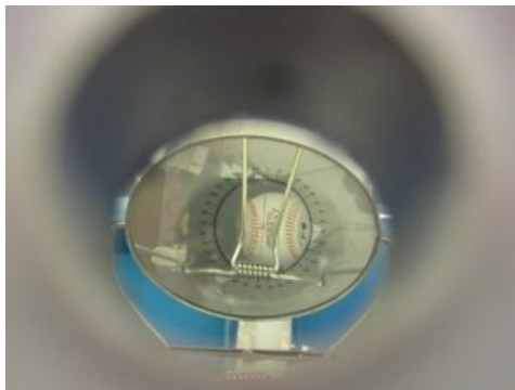
Fig. 2-7: View of the baseball from the viewing port.
