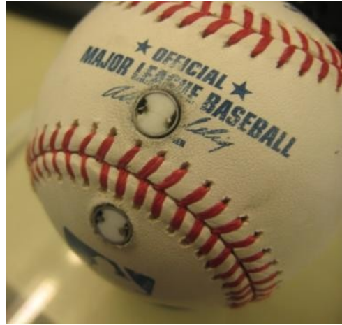
Fig. 2-30: Photo of the hot films before and after a seam. Data was recorded for two different rotation directions to test if the second seam affected the shear stress at both locations.
