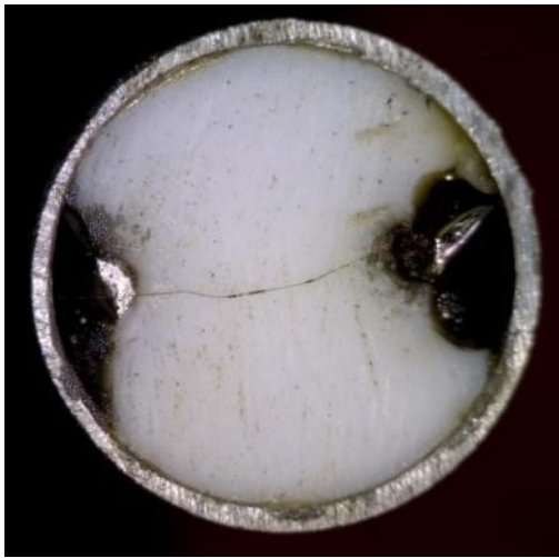
Fig. 2-22: Photomicrograph of 14.3 Ohm hot film in baseball. (Hot film 1)
