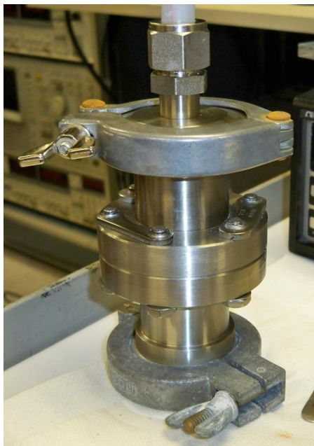
Figure 4.2-3. PCB and chip loaded into stainless steel vessel for calibration.
