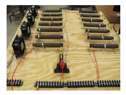
Figure 3.7: Resistance board for providing the winding short-circuit fault.
