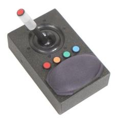
Figure 2.4, Diagram of MR compatible joystick.
