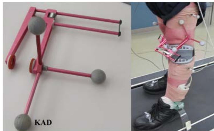
Figure 16: KAD (left) positioned over the femoral epicondyles during a static trial (right).
