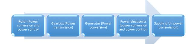
Fig. 1 .5: Basic power conversion wind turbine system [4].
